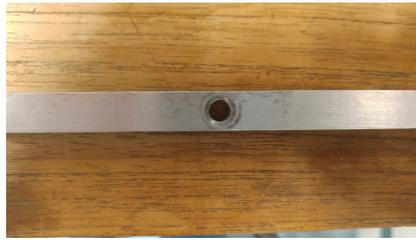
Figure 7.1: Plastic deformation caused by bearing stress in the fatigue test
