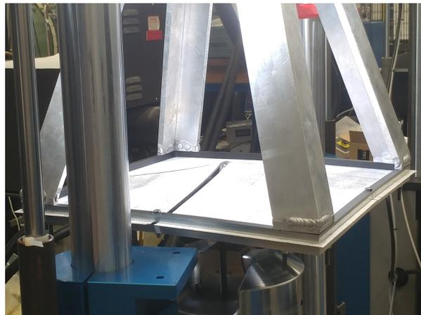
Figure 8.6: At the peak load the clamping frame starts to elastically bend with the specimen
