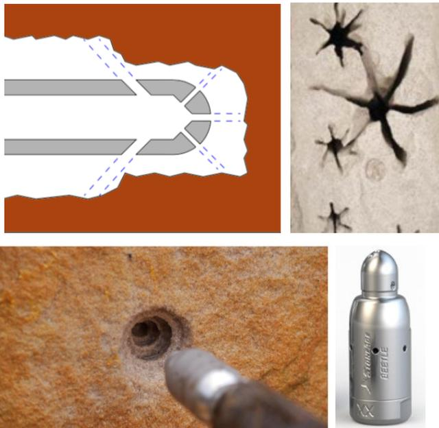
Figure 1. RJD holes and nozzles: Left to right (top): principal of forward and backward thrusters in static nozzle, star-shaped profiles in soft limestone with unconfined rock and static nozzle. Left to right (bottom): conical stop-start geometries formed at head of rotating nozzle; detail of Beetle, BT 18 mm rotating nozzle available from “StoneAge” used in true-triaxial laboratory tests performed at TUDelft.
