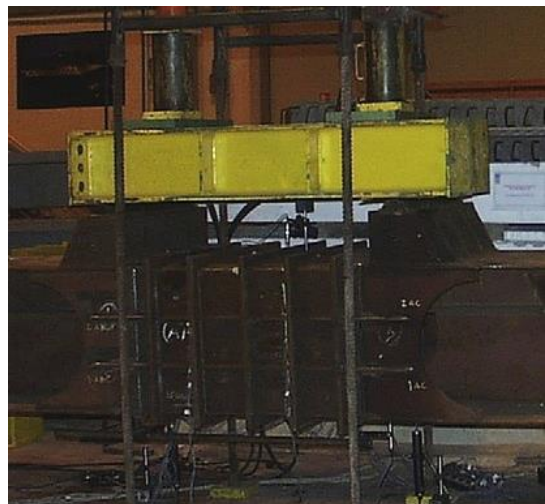
Fig. 1 Test setup of the box girder including part of the supporting structure and the loading device.
