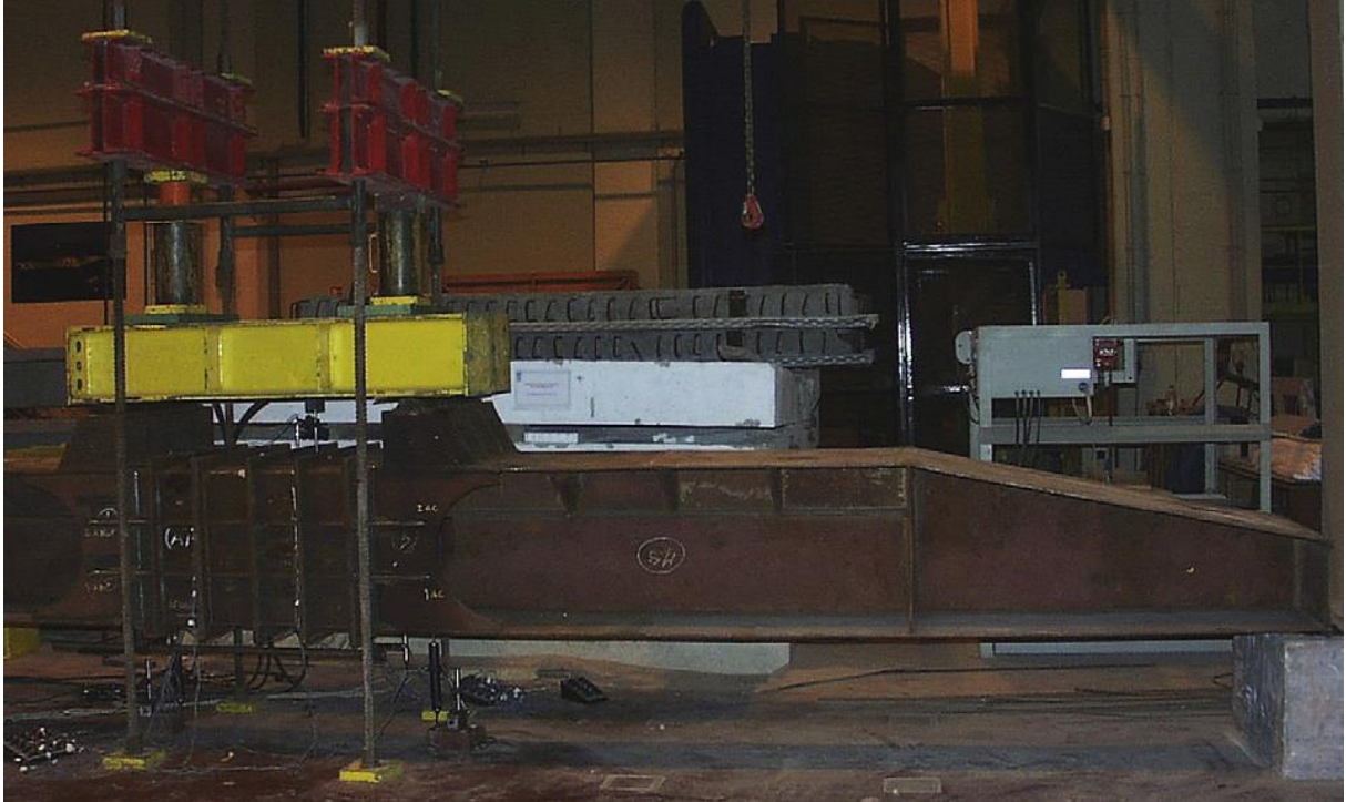
Fig 6.3 Test setup of the box girder H200 including part of the supporting structure and the loading device. [32]
