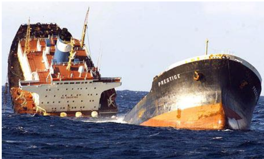
Fig 2.1 The hull of the Prestige has buckled after first damage which caused severe flooding and thus made the construction overstressed by the flooded load condition.
