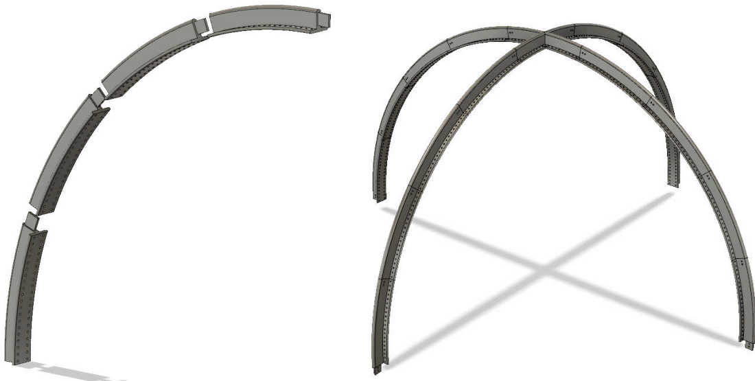
Figure 5.2: Model of the 3D printed segments which are interlocked to make an arc, as shown on the right.
