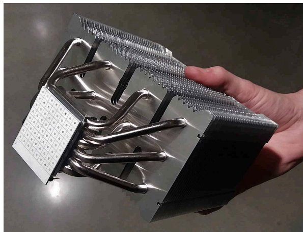
Figure 1.2: Example of a phased array antenna for 5G applications. Currently being developed at TU Eindhoven.
