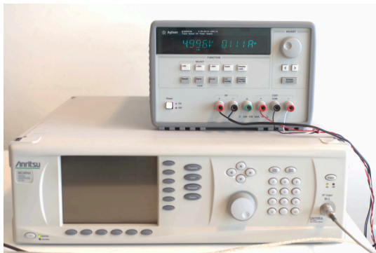
Figure 5.9: Signal generator used for AUT signal generation. On top, the power supply for the amplifier is visible.
