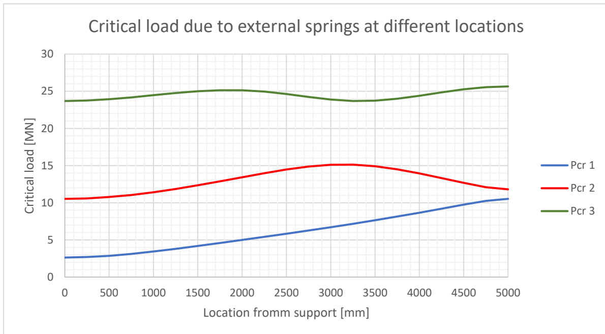
Figure 48: Effect of critical loads due to a single external spring at different distances from left pin support of a 10 000 mm simply supported column.
