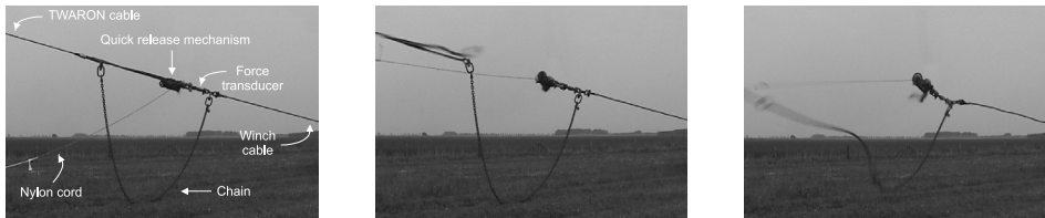
Figure 4.14: Step-relaxation hardware and recorded release. Left photograph: position of the TWARON cable, quick release mechanism, nylon cord, chain, force transducer, and winch cable at T = 0.0 s, middle photograph: position at T = 0.08 s, and right photograph: position at T = 0.16 s.
