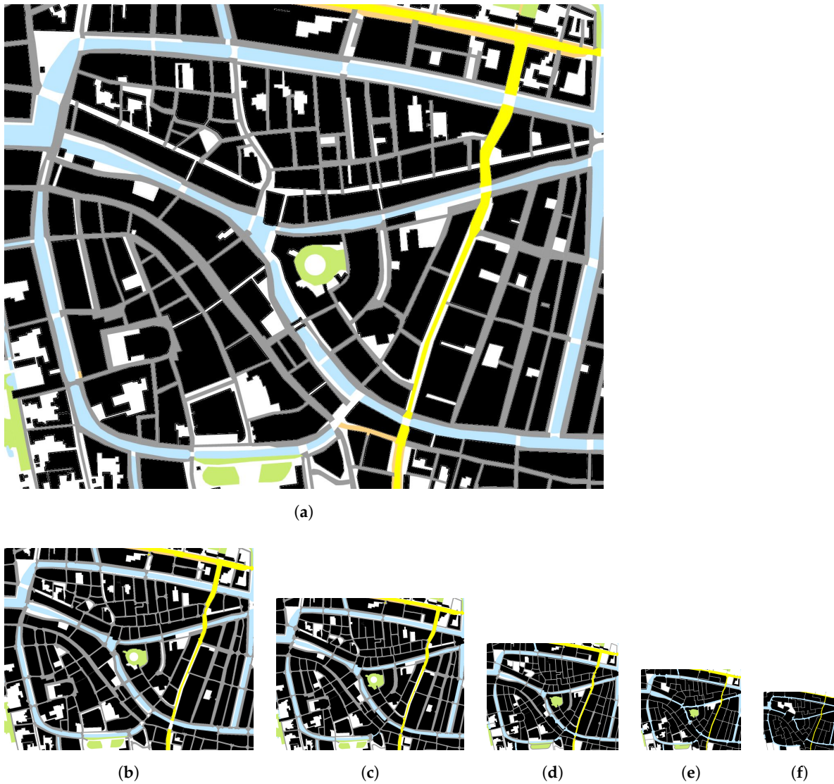
Figure 9. (a–f) An example of the generalization process for the city center dataset. (a) shows the input; The other subfigures (b–f) represent 60.6%, 68.7%, 80.8%, 88.9% and 95.0% of the process, where 0% is the input with 19,400 faces and 100% is one face. Note: the map fragments are displayed at the intended target scales; (a) 1:10 k; (b) 1:16 k; (c) 1:18 k; (d) 1:23 k; (e) 1:30 k; (f) 1:45 k.
