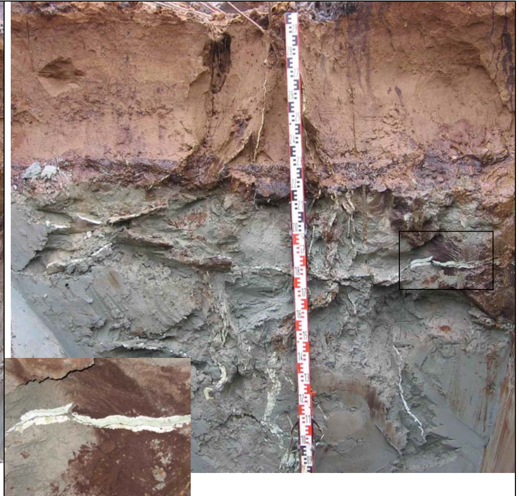
Figure 7.3b. Close up cross-section B-B, -0.9 m to -2.5 m below ground level. Resin discs generally in horizontal and vertical direction sometimes consisting of stacked discs from the first and second injection, see cut out.
