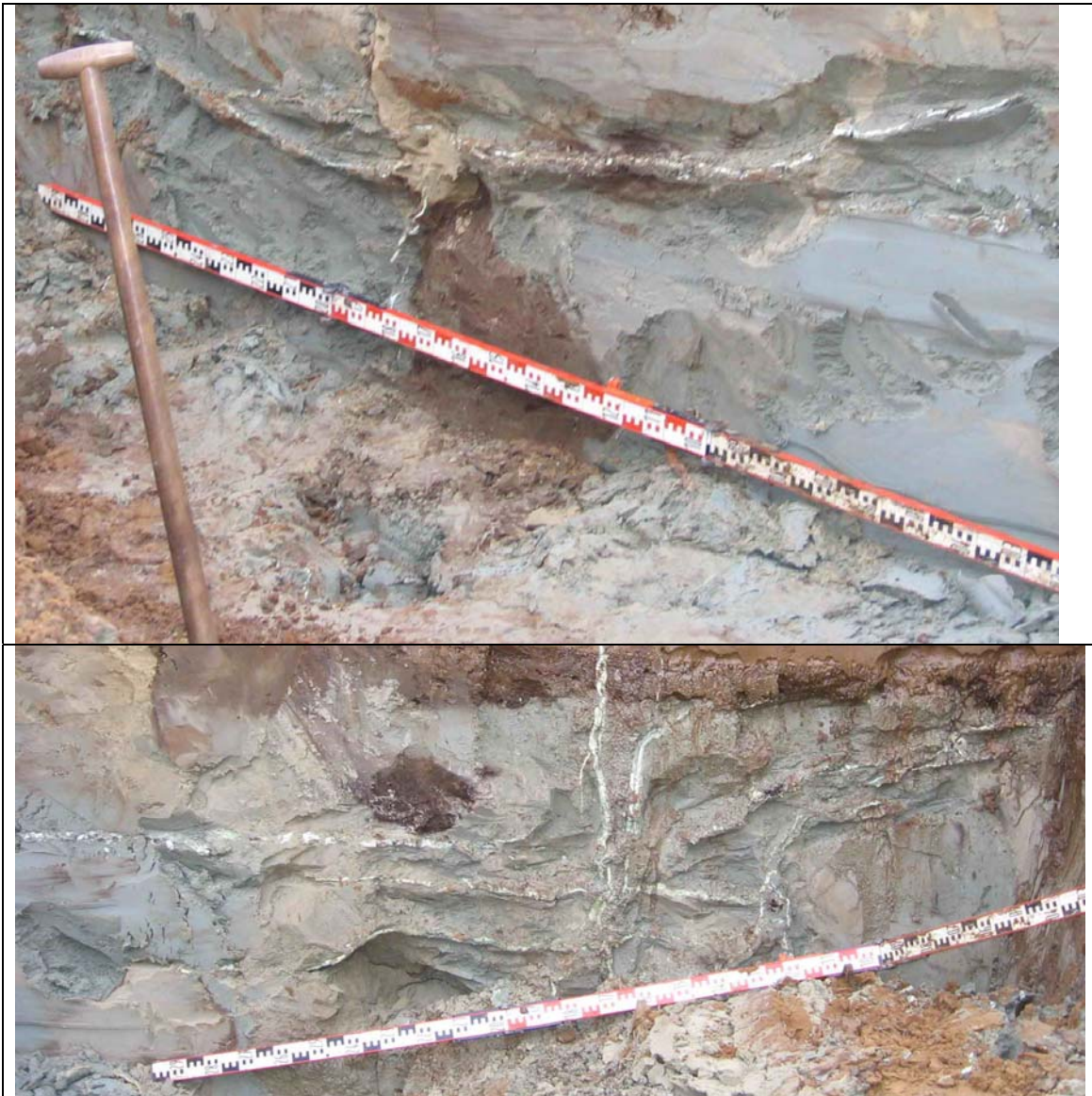
Figure 7.8. The horizontal resin discs have a maximum width of about 2.5 to 3 meters. The injection point being near the middle of the disc.
