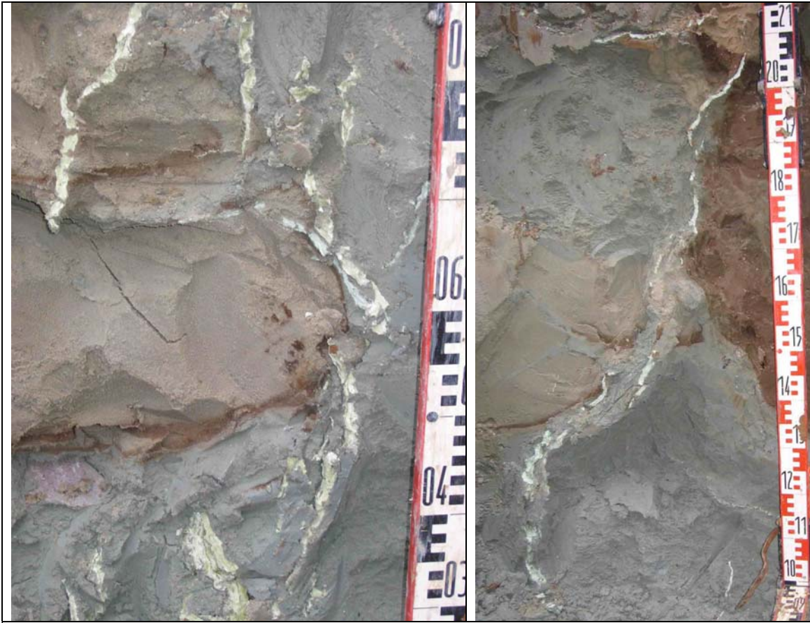
Figure 7.7. The resin takes the way of the least resistance; along the borders of two different soil types in the weakest soil.
