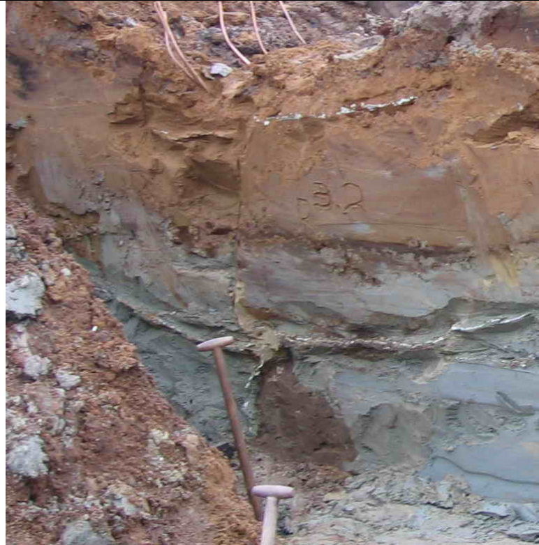
Figure 7.5. Part 3.2, Cross-section D-D, -0.6 m to -2.8 m below grade. Two horizontal and a vertical resin discs. This strip is injected under once.
