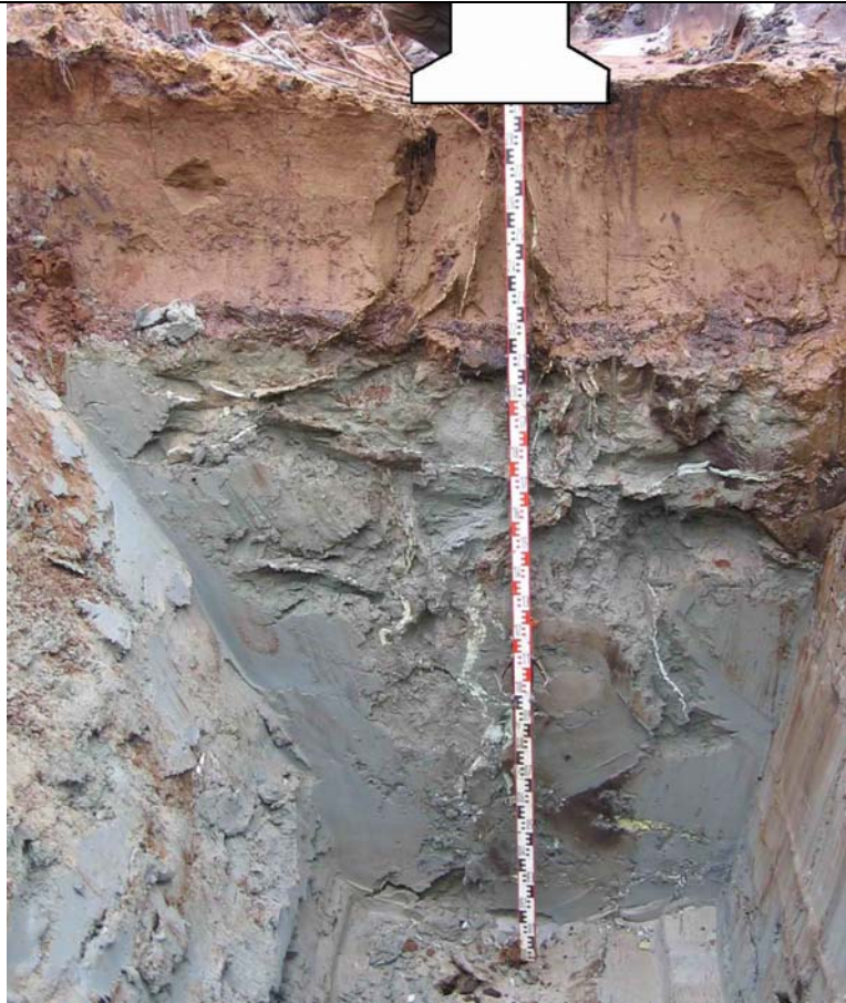
Figure 7.3a. Part 3.4, Cross-section B-B, under strip foundation -0.6 m to -3.4 m below grade; drawn injection.
