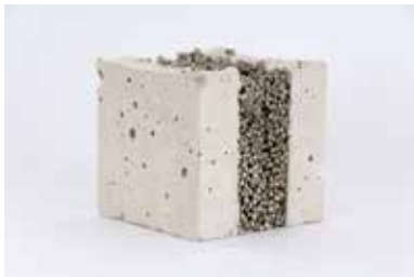
Figure A20 - Two types of concrete casted with 30 minutes in between.
