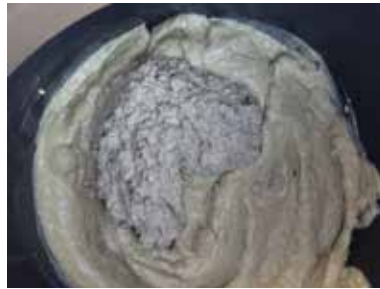
Figure A9 (left) - Concrete with bentonite as support material
