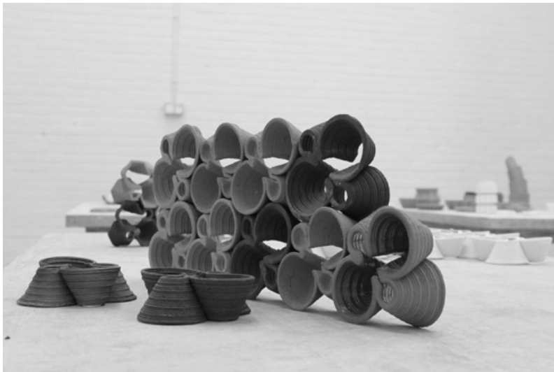
Figure 71 - 3D printed clay elements (1)
