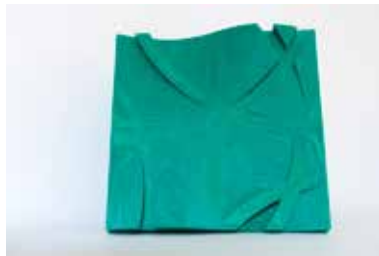
Figure A3 (left) - Part of the mould printed out of ABS
