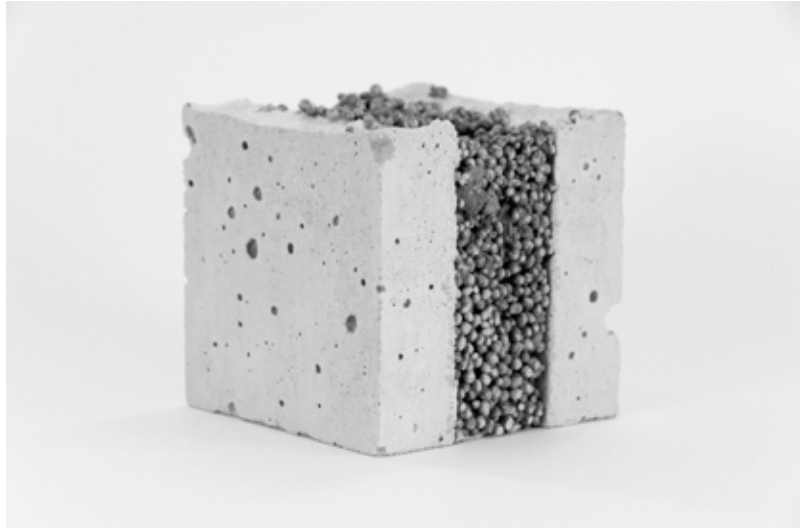
Figure 105 - Concrete core with expanded glass balls
