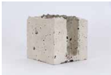
Figure A19 (right) - Two types of concrete casted with 30 minutes in between
