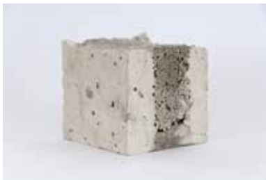
Figure A18 (left) - Two types of concrete casted at once
