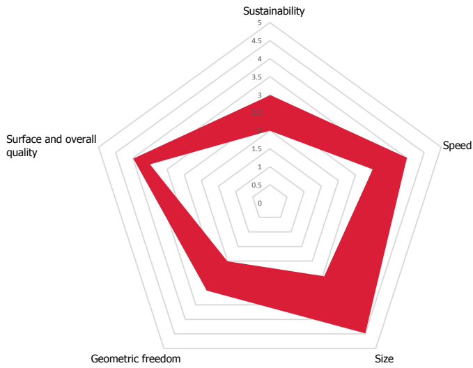
Figure 78 - Characteristics of CNC milling of concrete
