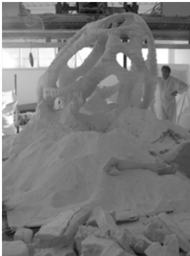
Figure 49 - D-Shape removing the material that has not been bound (1)
