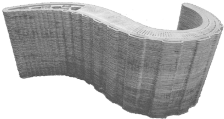
Figure 45 - Bench made with 3D-Concrete printing (1)
