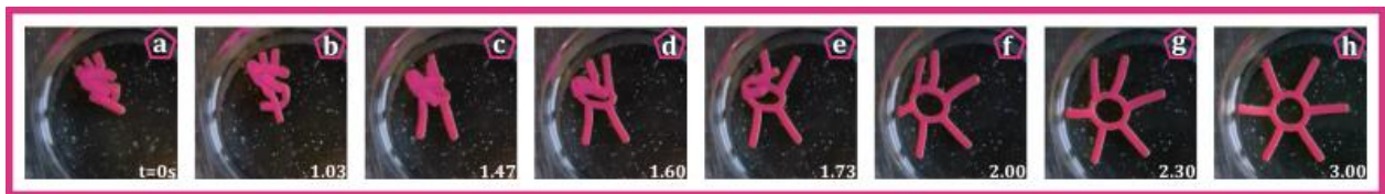
Figure 2-3: Recovery of a crumpled element to its permanent 2D shape in time, when submerged in water with a temperature of approximately 95°C.
