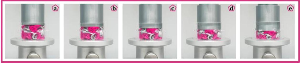
Figure 2-5: Different stages during the mechanical compression testing
