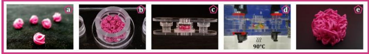
Figure 2-4: The process of creating a scaffold a . Multiple crumpled elements b . a specific number of crumpled elements were placed in a cylindrical holder c . The holder was closed with a top lid. In the holder, there are multiple holes to let the hot water flow through d . The holder was placed in a hot water bath of 90°C for 15 seconds e . After the scaffold was cooled down this is the end product.
