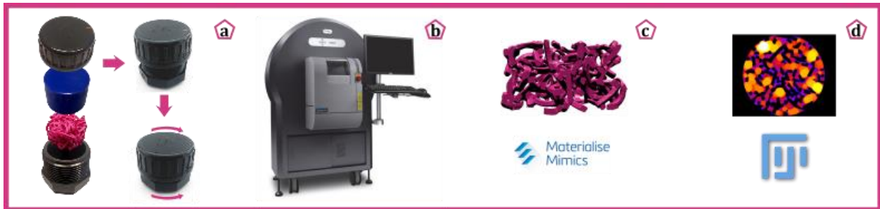
Figure 2-6: a. device used to manually compress the crumpled-based scaffolds in between scans b. Quantum FX micro-CT imaging system used for the non-destructive scanning of scaffolds c. Materialise Mimics software was used to render and reslice the Dicom files obtained by scanning the scaffolds with the micro-CT scanner d. Fiji ImageJ software together with the plugin BoneJ was used to define the morphological properties of the scaffolds.
