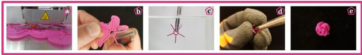
Figure 2-2: The process of creating a crumpled element a. Printing the elements with a FDM printer b. postprocessing the elements by removing the brim layer c. Heating the element by holding it in a waterbed of 90°C for 10 seconds d. crumpling the element by hand.
