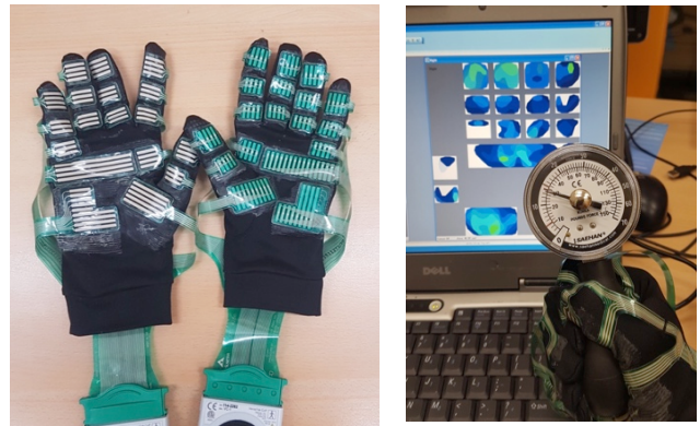
Figure 3. left: Tekscan pressure sensors attached on thin gloves, right: output of the pressure sensor visualized
