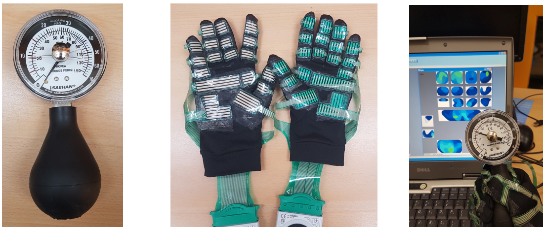
Figure C-1 Left: hand dynamometer, middle: gloves with Tekscan sensors, right: raw sensil output while applying a force to the hand dynamometer
