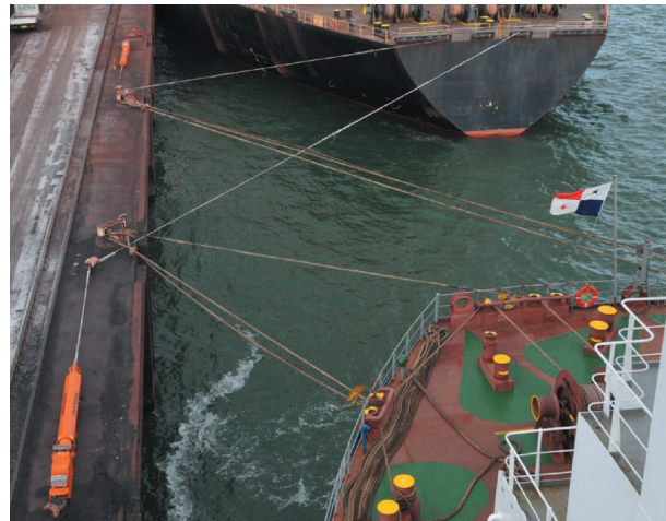
Figure H.3: ShoreTension (left hand) implemented at a harbor quay side. source: ShoreTension brochure [47]
