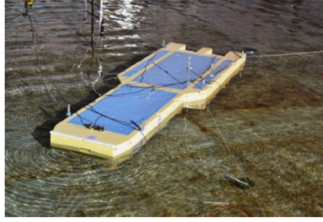
Figure 5.3: Snapshot of the barge shape used for comparing RAOs of Iron Lady source: Motion responses of a moored barge in shallow water. [27]
