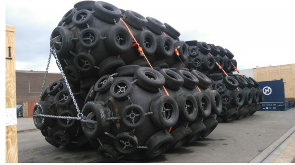
(b) Three Yokohama fenders oriented as triangle to double vessel spacing.
