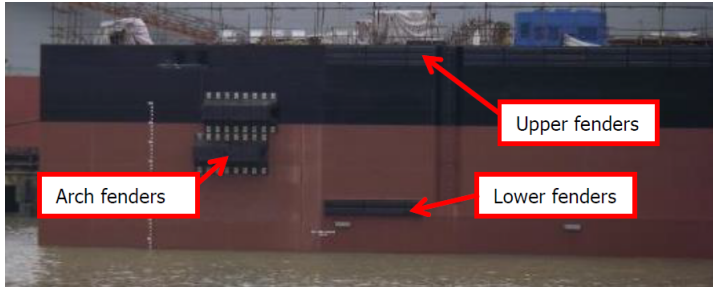
(a) Fenders fixed t Iron Lady with a thickness of 0.3 m
