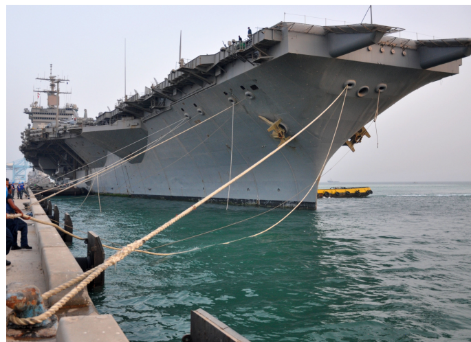
Figure H.1: Aircraft carrier with mooring lines going inside the hull.
