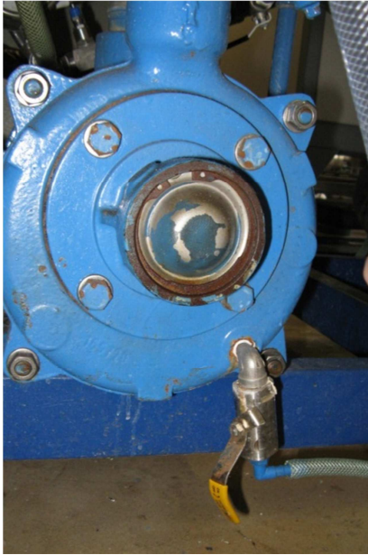
Figure M.20. Yellow tap at the bottom of the pump to empty the vacuum pump.
