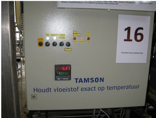
Figure M.7. The cooling machine. The most left button turns on the cooling liquid pump and the one next to it the compressor.
