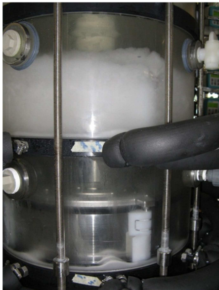
Figure 4.8. Salt accumulates atop and around the upper heat exchanger.
