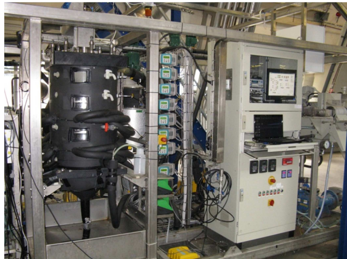
Figure 4.2. An overview of the 200 liter pilot plant. The insulated crystallizer is shown at the left. Samples can be drawn from the top middle and bottom section of the crystallizer vessel.
