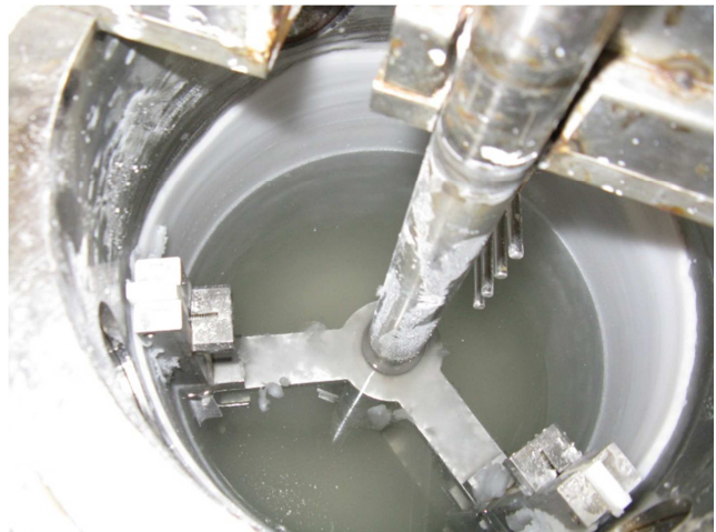
Figure 3.11. Scale grown on the wall of the 10 L scraped wall crystallizer. The starting solution was a pure 8 wt% \text{Na}_2\text{SO}_4 solution.
