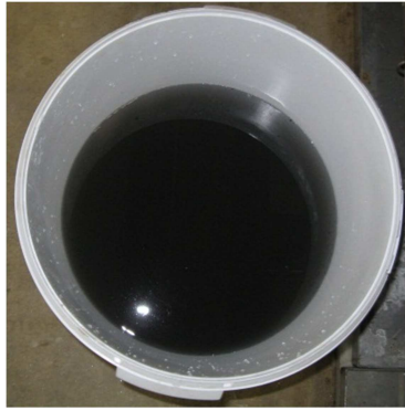
Figure 4.15. The color of the industrial \text{Na}_2\text{SO}_4 - solution after the crystallization experiment. Black solid particles are suspended in the liquid. \text{H}_2\text{S} gas is detected near the liquid surface.
