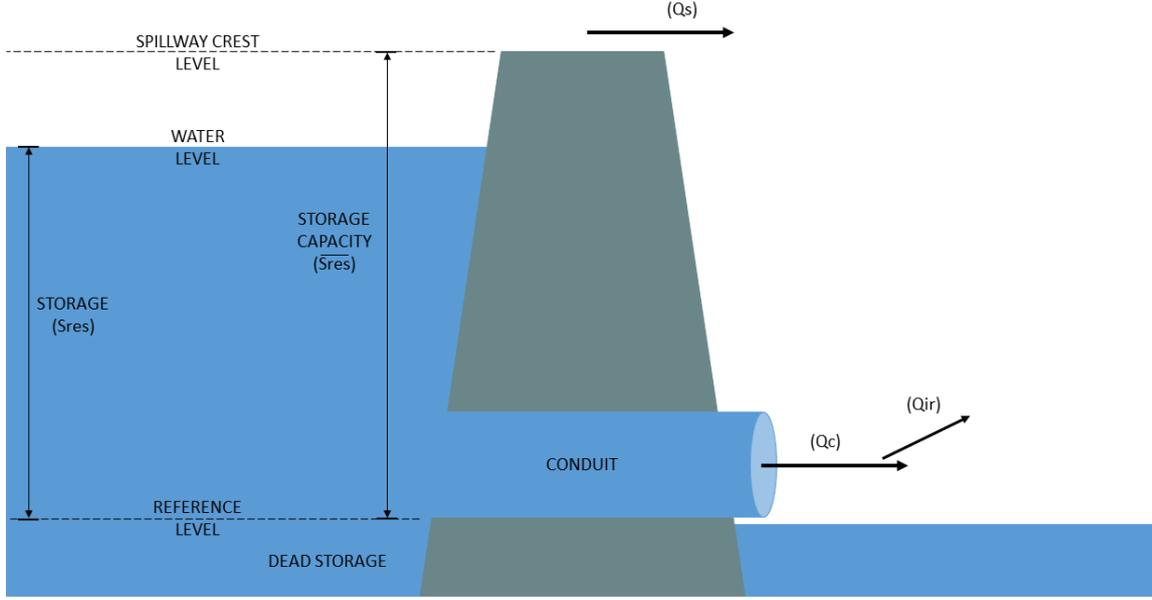
Figure 3.1: Schematic representation of a reservoir with overflow spillways.
