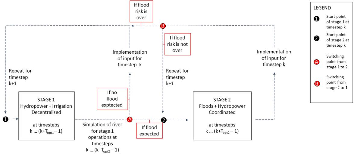
Figure 4.2: Schematic representation of the two-stage MPC method.
