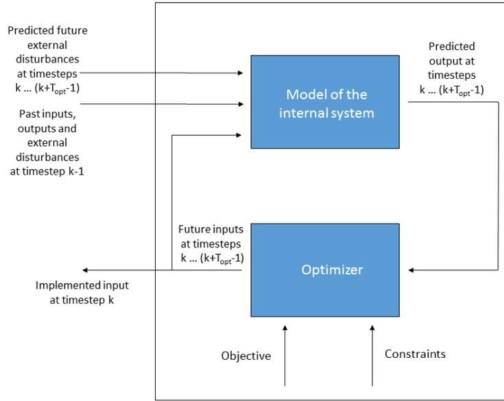
Figure 4.1: Structure of the MPC method performed on timestep  $k$ .
