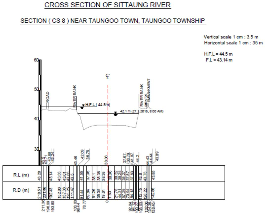
Figure 3.2: Cross section measurement of the Sittaung river near Taungoo town (Rest, 2015)
