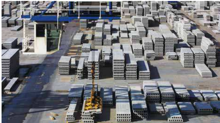
Figure 2-16: Stock of hollow core slabs in a storage hall (Source: BFBN)
