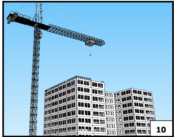
Use a building crane to take out the wall elements
