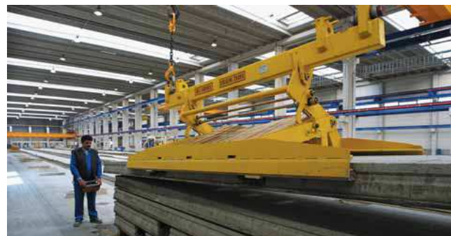
Figure 2-11: Bucket to clasp the hollow core slabs (source: BFBN)
