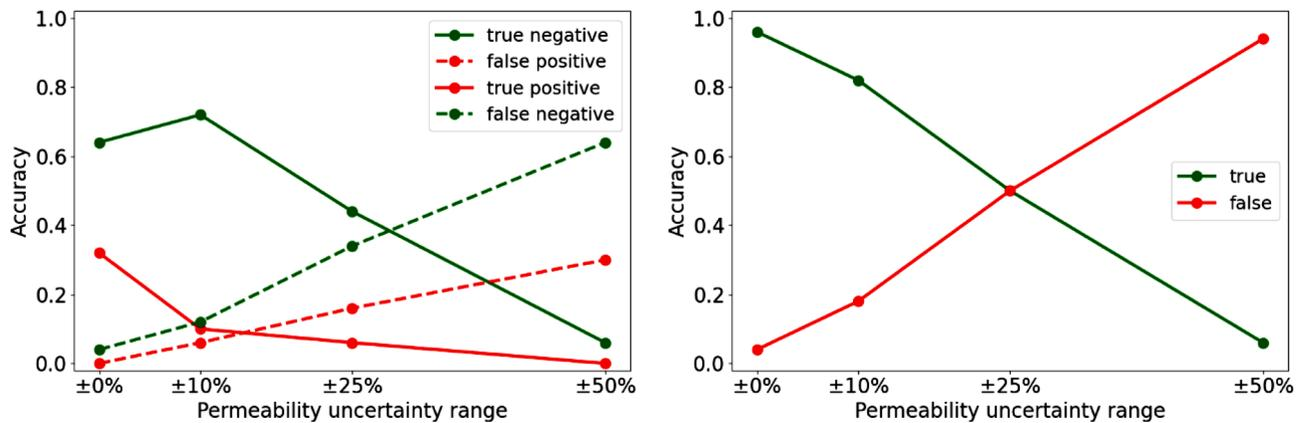
Fig. 21. Accuracy of conformance assessment as a function of the uncertainty range on the permeability of the first layer of the Smeaheia model: fraction of true and false statements for a BHP monitoring duration of 15 years including also uncertainty on connectivity to depleting Troll field.
