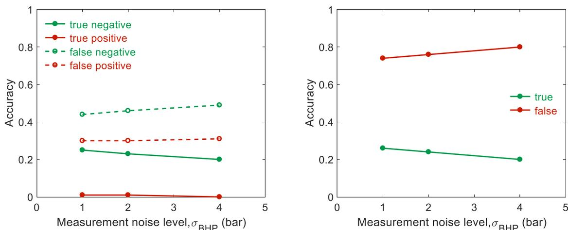
**Fig. 6.** Accuracy of conformance statements for different levels of noise in BHP measurements: fraction of true and false positives and negatives (left) and true (accurate) and false (inaccurate) assessments (right). In this and other experiments described in this section,  $p_\alpha = 1$ .
