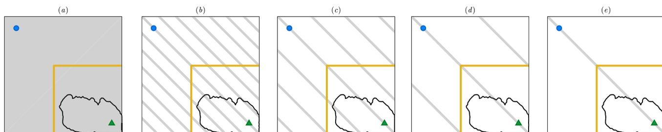
Fig. 12. Five survey configurations with different degrees of sparsity. The grey pixels indicate the locations (grid blocks) in the reservoir where the CO<sub>2</sub> plume can be tracked. The positions of the CO<sub>2</sub> injection and brine production wells are indicated by the green triangle and blue circle, respectively. (For interpretation of the references to color in this figure legend, the reader is referred to the web version of this article.)
