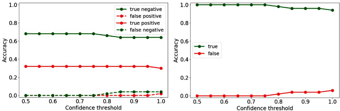
Fig. 19. Accuracy of conformance assessment as a function of the confidence threshold ( $p_\alpha$ ): fraction of true and false statements for a BHP monitoring duration of 15 years in the presence of uncertainty in connectivity to the neighboring depleting field.
