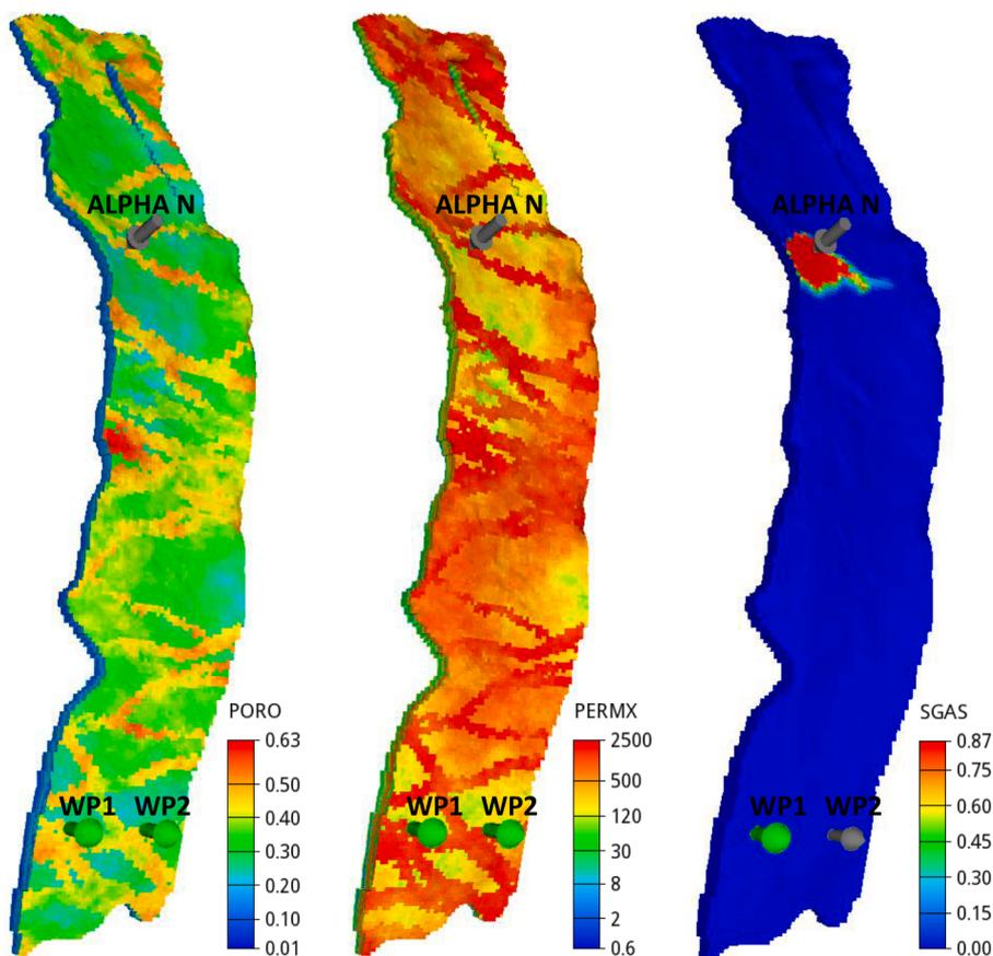
Fig. 14. Top view of the Smeaheia reservoir model: porosity (left) and permeability (middle) fields and CO<sub>2</sub> plume at the end of the simulated period (right). CO<sub>2</sub> is injected in Alpha structure and connection to neighboring field in depletion is modelled by two artificial production wells in the southern portion of the model.
