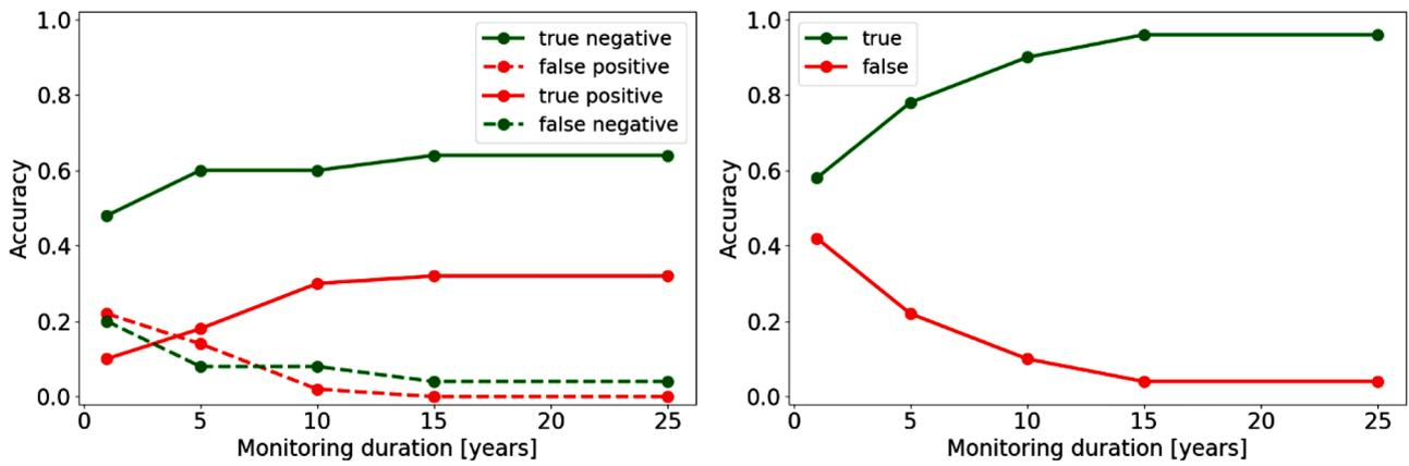
Fig. 18. Accuracy of conformance assessment as a function of the duration of BHP monitoring: fraction of true and false statements for a confidence threshold  $p_\alpha = 0.95$  in the presence of uncertainty in connectivity to the neighboring depleting field.
