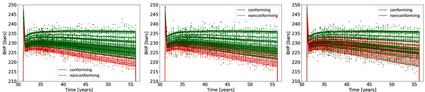
Fig. 20. Simulated BHP profiles and measurements at the CO<sub>2</sub> injection well for the Smeaheia case with varying connectivity to the depleting Troll field and increasing uncertainty on the permeability of the first layer of the model:  $\pm 10\%$  (left),  $\pm 25\%$  (middle) and  $\pm 50\%$  (right).
