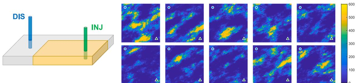
Fig. 2. Synthetic test case study with one CO<sub>2</sub> injection well and one brine discharge well (left). The yellow box indicates the region within the conformance boundary. 10 randomly selected realizations of the permeability field (right); the color bar indicates the permeability values in mD. (For interpretation of the references to color in this figure legend, the reader is referred to the web version of this article.)
