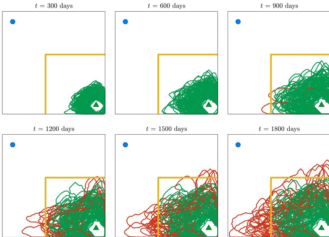
Fig. 4. Development of the CO<sub>2</sub> plume conformance over time based on simulation of the initial ensemble of model realizations (using the same color scheme as in Fig. 3).
