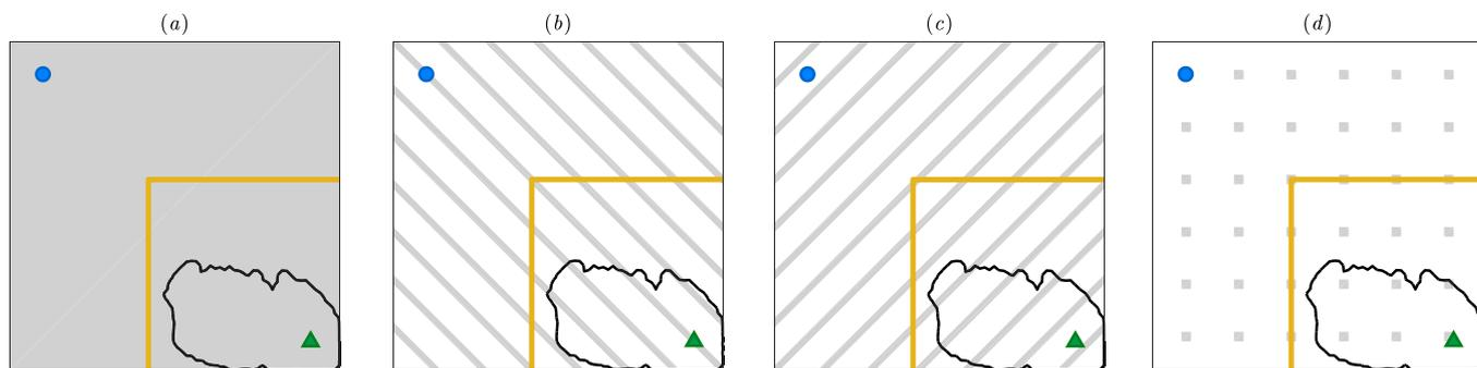
Fig. 10. Four survey configurations with different reservoir coverages or orientations. The grey area (a), lines (b and c) and pixels (d) indicate the locations (grid blocks) in the reservoir where the saturation can be observed. The positions of the CO<sub>2</sub> injection and brine production wells are indicated by the green triangle and blue circle, respectively. (For interpretation of the references to color in this figure legend, the reader is referred to the web version of this article.)
