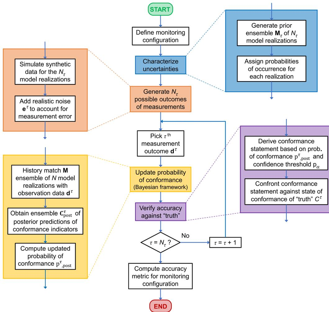
Fig. 1. Proposed workflow for quantifying the expected accuracy to be achieved with a candidate monitoring configuration.
