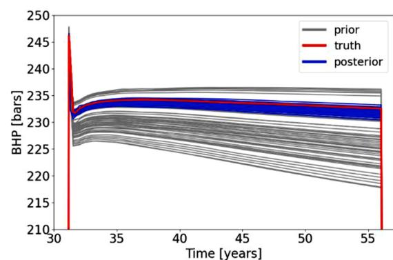
**Fig. 17.** Bottom-hole pressure predictions at the injection well as result of history matching of BHP measurements during  $T_{\text{BHP}} = 15$  years for one of the plausible truth realizations. Grey lines were obtained with the prior ensemble, blue lines with the posterior ensemble and the red line with the truth realization. (For interpretation of the references to color in this figure legend, the reader is referred to the web version of this article.)
