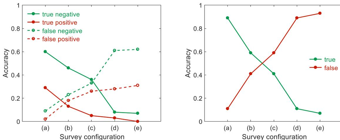
Fig. 13. Accuracy of conformance statements for the survey configurations from Fig. 12 with five different degrees of sparsity for a fixed orientation: fraction of true and false positives and negatives (left) and true (accurate) and false (inaccurate) assessments (right).
