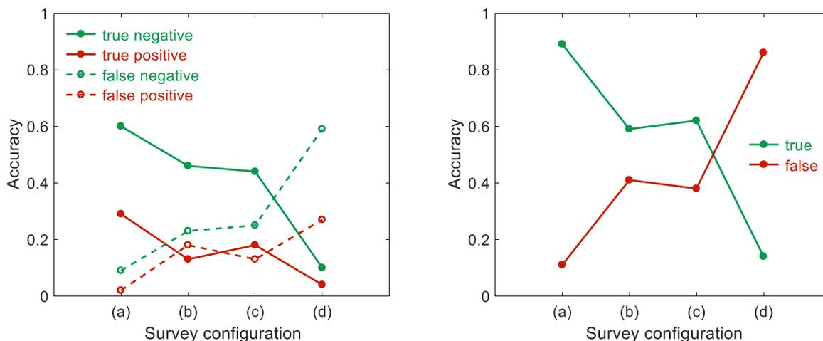
Fig. 11. Accuracy of conformance statements for the four different survey configurations from Fig. 9: fraction of true and false positives and negatives (left) and true (accurate) and false (inaccurate) assessments (right).
