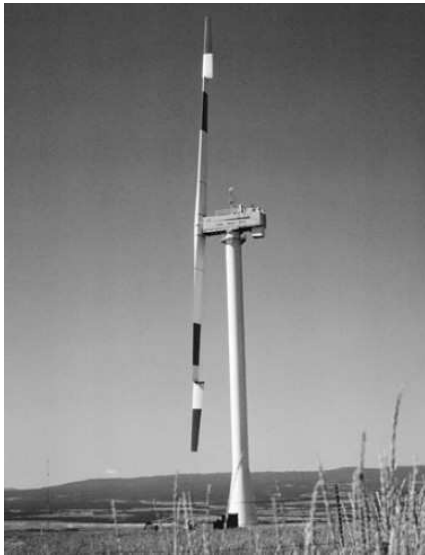
(c) MOD-2 wind turbine (1980) built by Boeing with a rotor diameter of 91 m and rated power of 2.5 MW.
