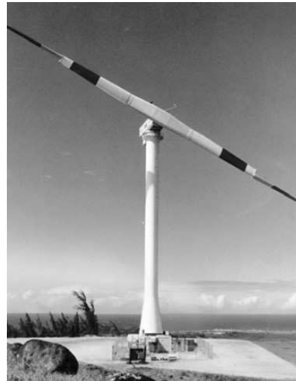
(d) MOD-5B wind turbine (1987) built by Boeing with a rotor diameter of 97 m and rated power of 3.2 MW.
