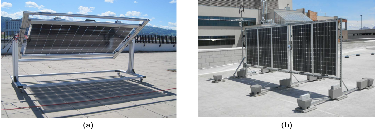
Figure 2.6: Ground shade condition in real experiment (a) a south facing and tilted module installation by Franhoufer [21] (b) and east-west vertical installation [13]. Note that the shaded ground area is larger in a tilted module (figure a).
