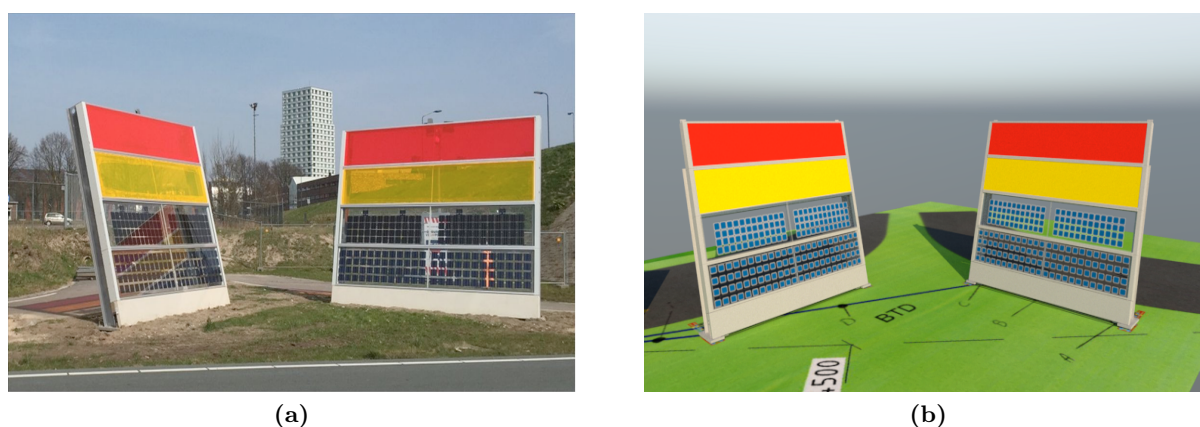
Figure 5.7: Comparison of SONOB Living Lab used for validation (a) Real condition [21] (b) Rendering of 3-D Drawing made in SketchUp. All the components and dimensions used in the 3-D model are exactly followed the real aspect given in the original technical drawing.
