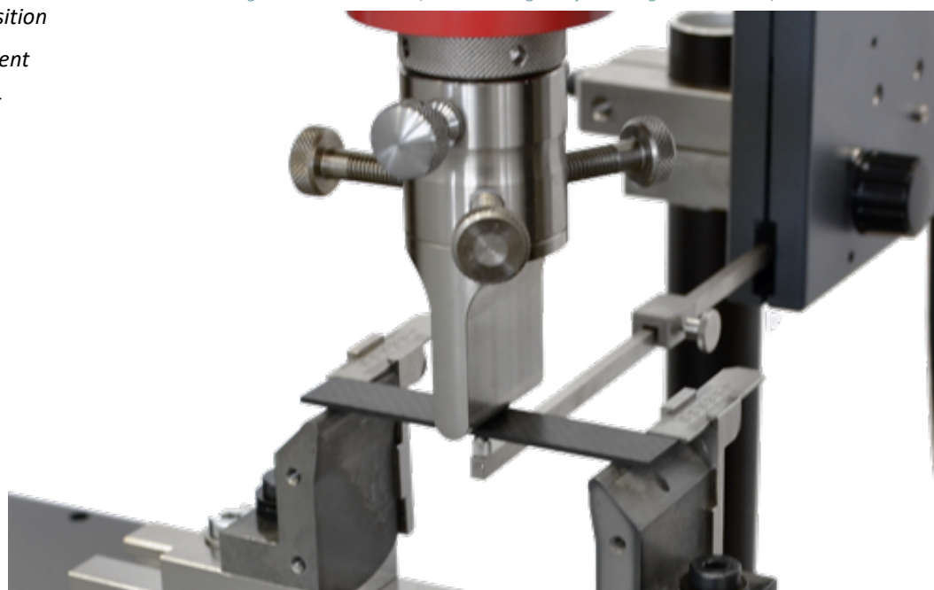
Figure 1.26: The three point bending test for Young's Modulus capture.
