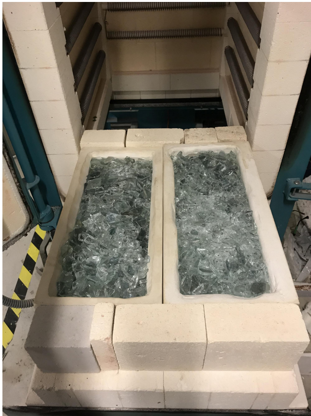
Figure 2.25: Mould with prepared glass mixtures before kiln-casting.
