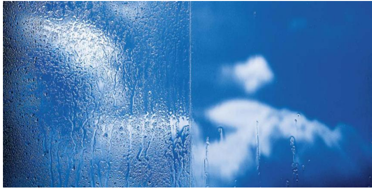
Figure 2.5: Coated glass. Glass coating mainly aiming at affect the transmission of glass, assisted in improve the glass appearance and surface condition. The coated glass is widely used as thermal control glass as well as self-cleaning glass.
