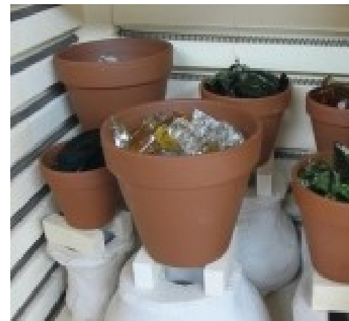
Figure 1.21: The kiln-casting with flower pot, placed on top of the mould, as a container for glass cullets; the left figure shows the glass melting process during casting; the right figure present the situation before casting.
