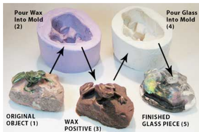
Figure 1.24: The lost wax mould.
