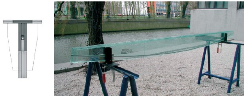
Figure 3.2: The cross section (left) and the prototype (right) of T-section beam, from [40].
