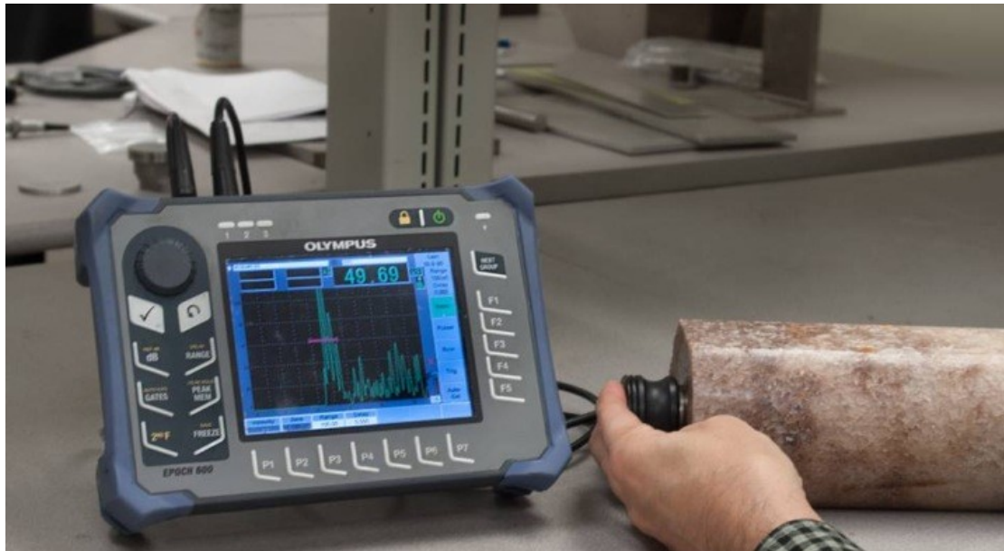
Figure 1.29: Ultrasonic velocity measurements in geological samples from Olympus company.
