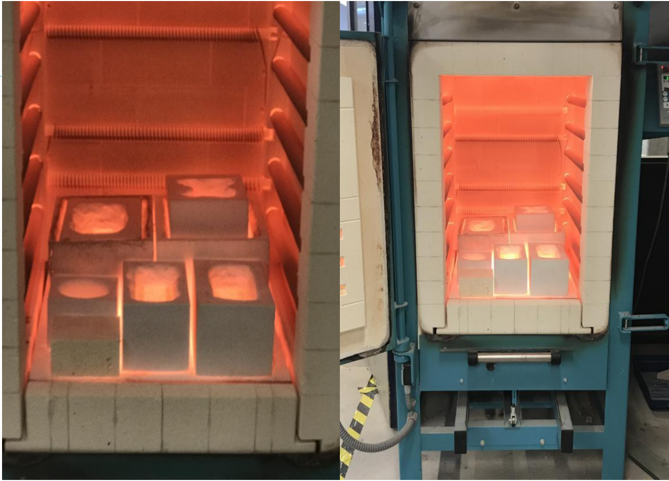
Figure 2.13: The manual quenching process during kiln casting.
