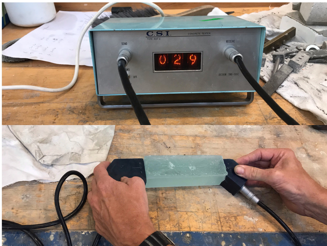
Figure 2.26: The ultrasonic method for Young's modulus testing, photo by author.
