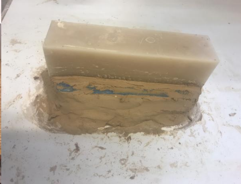
Figure 2.10: Wax model. Two finished wax models with corresponding rubber moulds shows in left sub-figure, while the right sub-figure presents the fixed wax model above a plastic base before crystal-cast mould fabricating.
