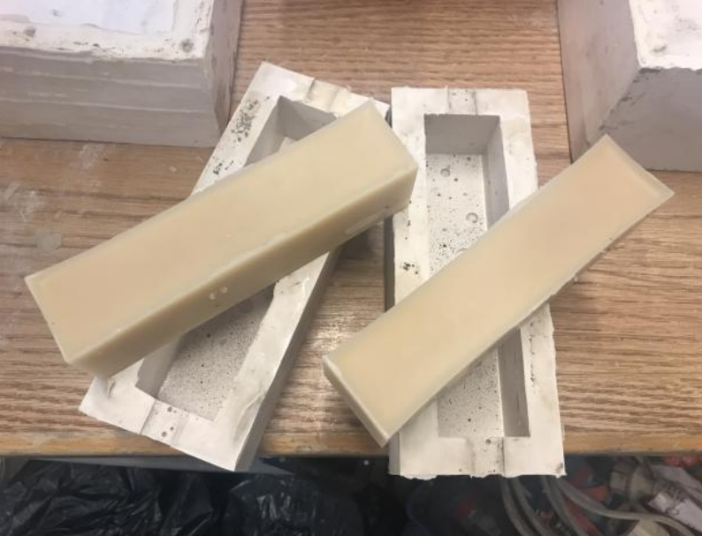
Figure 2.10: Wax model. Two finished wax models with corresponding rubber moulds shows in left sub-figure, while the right sub-figure presents the fixed wax model above a plastic base before crystal-cast mould fabricating.
