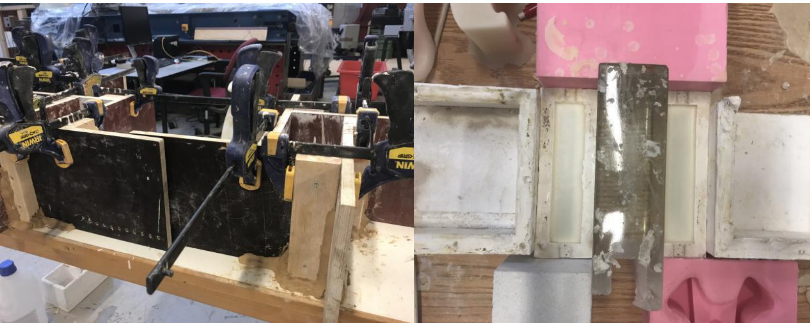
Figure 2.9: The production process of rubber mould. The left sub-figure shows rubber mould while curdling, with wooden panel and clay as fixer. On the right side is the finished rubber mould, which are well-placed before making wax mould.
