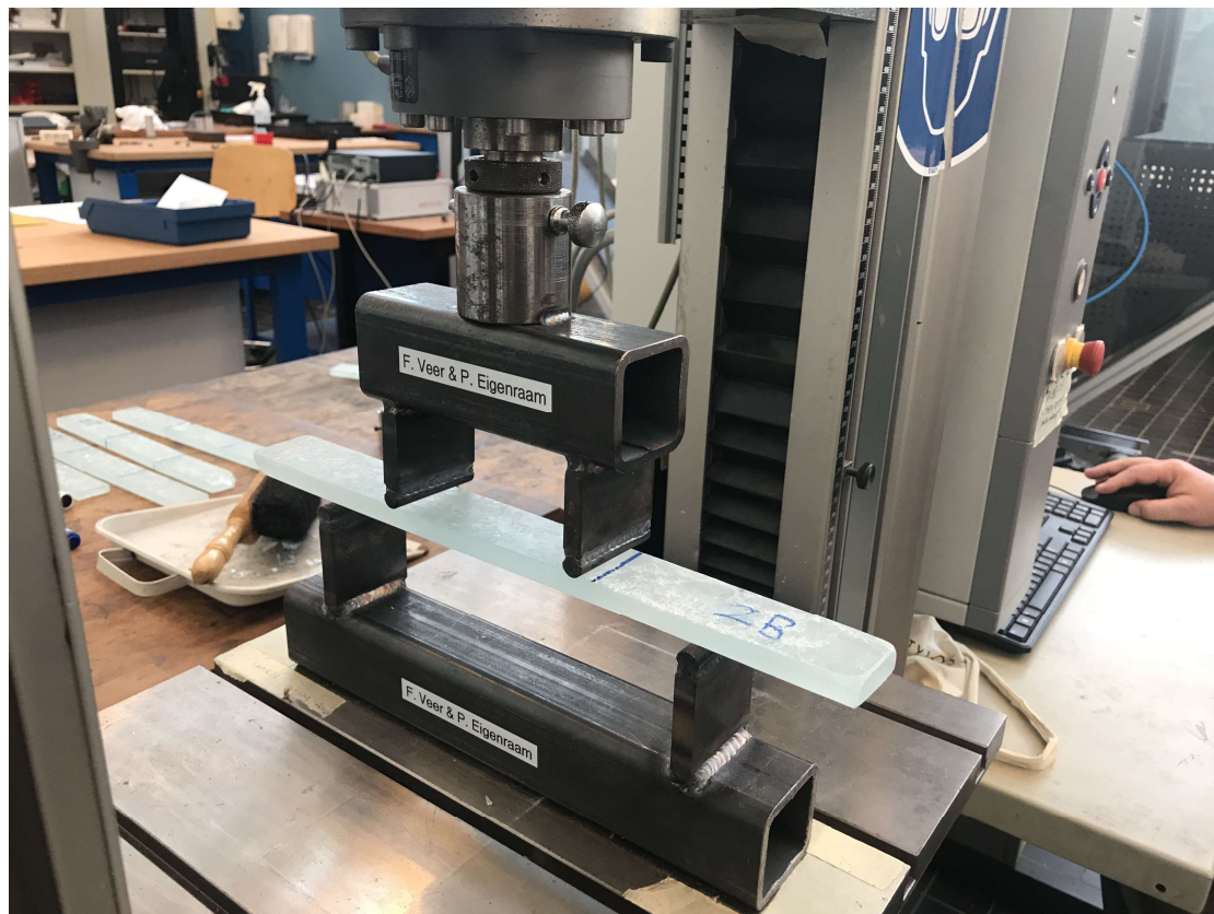
Figure 2.33: The four-point bending test of recycled glass beam, photo by author.
