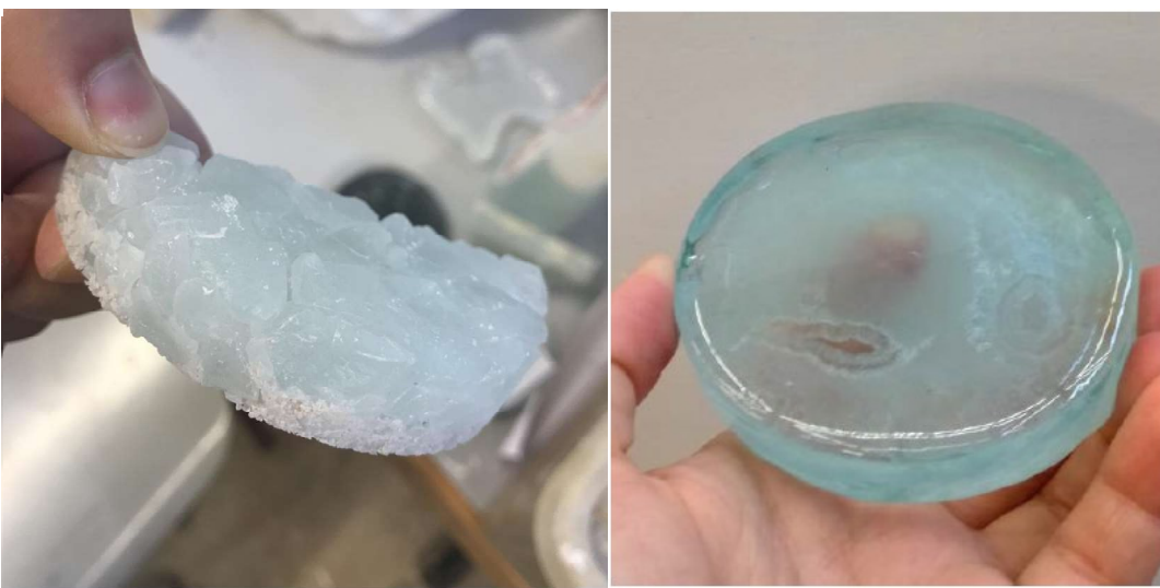
Figure 1.22: the float glass recycling through kiln-casting method, in 900 degrees (left) and 1250 degrees (right).
