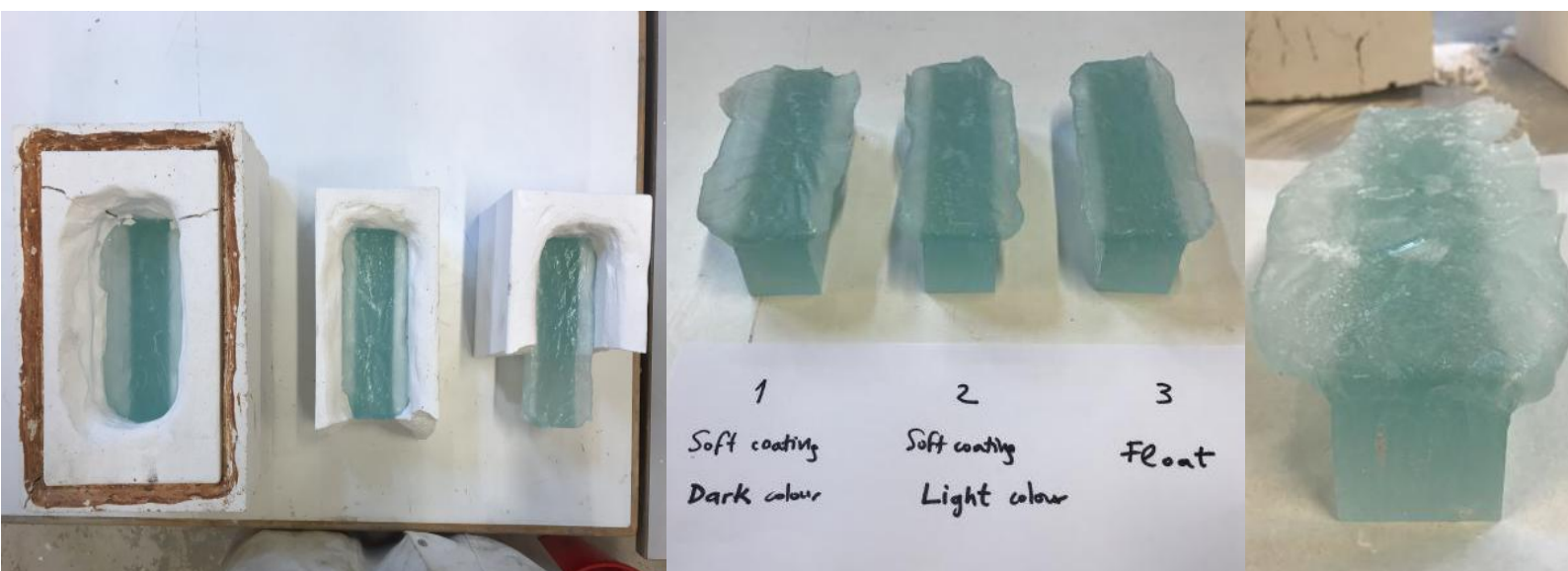
Figure 2.16: The recycled glass samples after kiln-casting. On the left are three glass samples taken out of the kiln, covered by the mould; the middle sub-figure shows glass samples without mould in correspond to their category, the right sub-figure shows the recycled hard coating samples.
