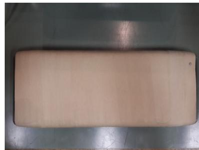
**Figure 3-5:** Substrate wrapped with Crêped presspaper
