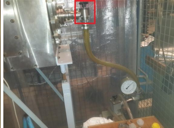
**Figure 4-9:** Test tank to vacuum pump connection with tank air outlet valve marked
