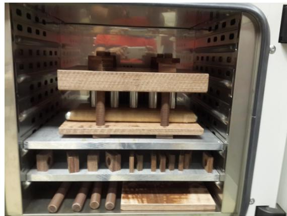
(b) Assembled frame kept for drying
