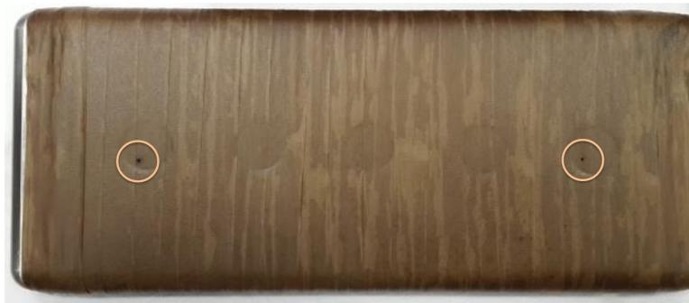
**Figure 5-23:** Punctures in sample bar 9 caused by the breakdown events
