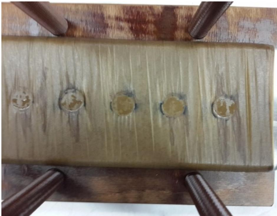
**Figure 5-26:** Carbonization caused by heavy discharges on sample bar 11
