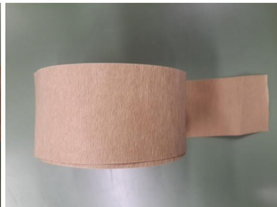
**Figure 2-2:** Thermally upgraded crêped presspaper
