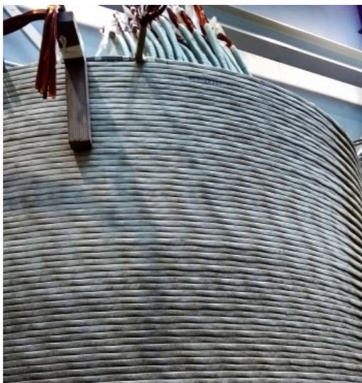
**Figure 2-4:** Front view of a winding (Courtesy: Royal SMIT)
