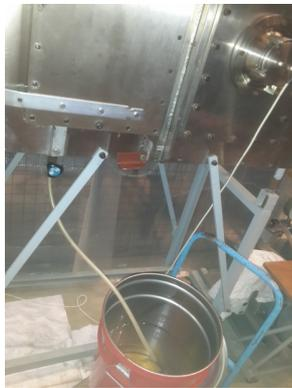
**Figure 4-13:** Oil filling in progress
