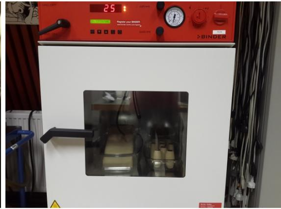
**Figure 5-2:** Paper samples placed in the vacuum oven (10 mbar (abs.), 25 °C)
