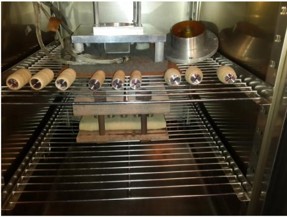
**Figure 5-1:** Paper samples placed in climate chamber
