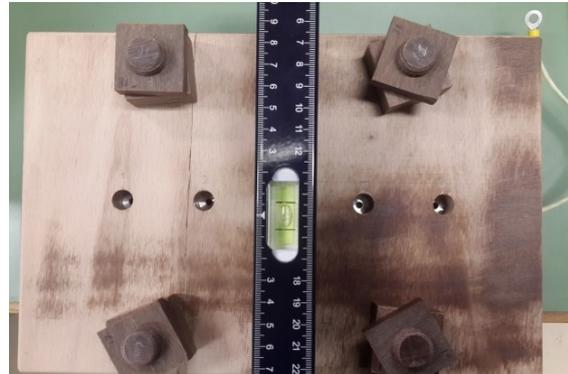
**Figure 3-11:** Level check performed while setting clamping force
