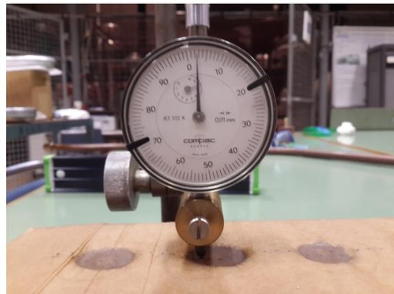
**Figure 5-29:** Measuring depth of the depression using a dial gauge
