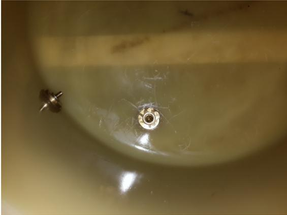
**Figure 4-8:** Oil filling and draining port (centre) and stud for connection of test object to earth (left)
