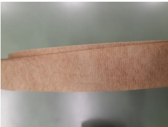
**Figure 2-1:** Thermally upgraded presspaper
