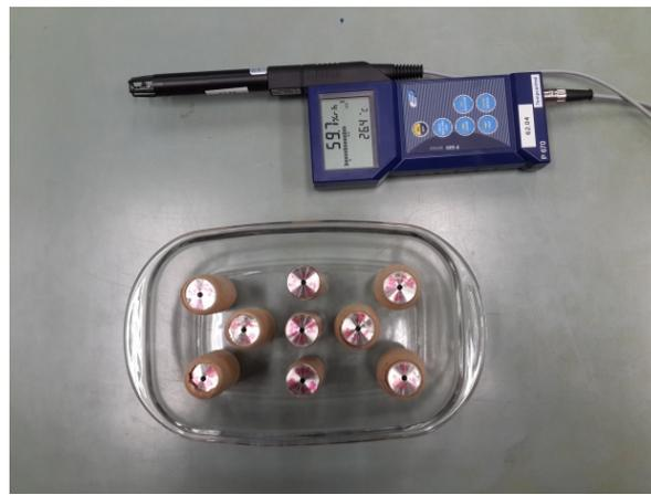
Figure 5-5: Samples placed in ambient conditions after vacuum cycle
