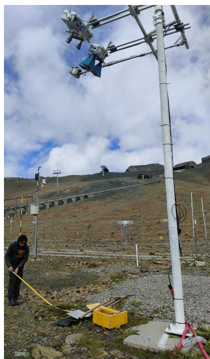
Figure 15. Field setup of the shovel-detection test.
