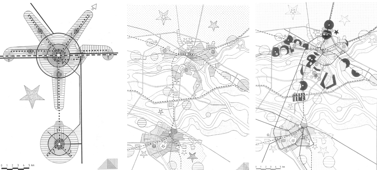
Fig.5-38 The normative theoretical model chosen for the twin cities Arnhem-Nijmegen (left) (see Fig.6-12.1-7) leads via a confrontation process with a model of the existing situation (centre) to a development model for these two cities (right) (Scholten 1992: 110; 141; legends omitted) (see also Section 6.4.1).
