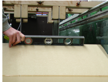
Figure 6.29: Plate levelled using a plumb rule
