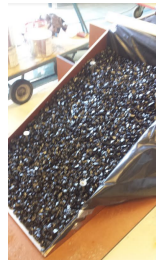
Figure B.04: Mold for total core, slope placed as well
