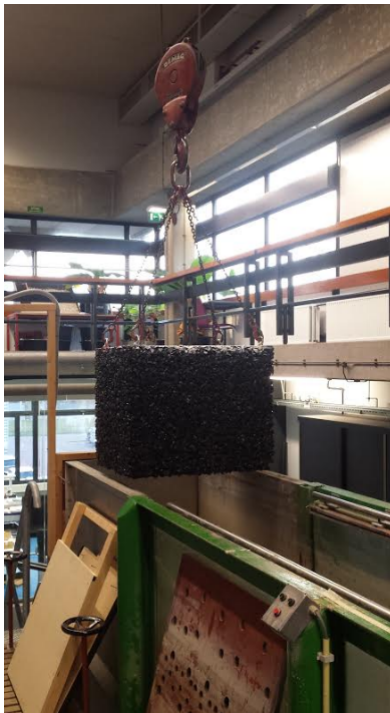
Figure B.05: Centre part of the core is placed in the wave flume
