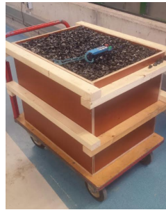
Figure B.02: Centre part of the core constructed in the mold
