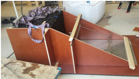
Figure B.03: Mold for total core, centre part is already placed
