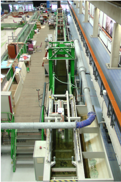
Figure 6.2: Overview of the wave flume
