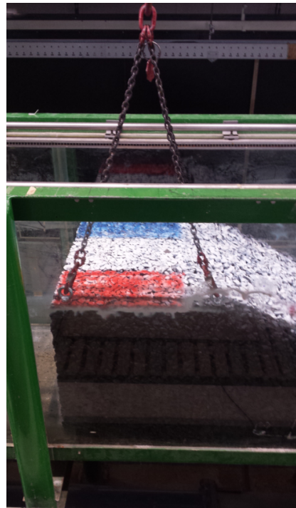
Figure B.06: Centre part of the core is removed from the wave flume
