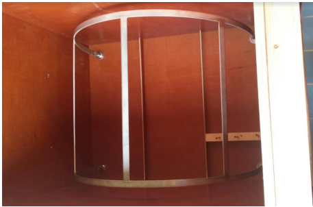
Figure B.01: Top view: Mold in which centre part is constructed.
