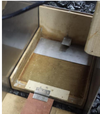
Figure 6.25: Crown wall connected to a hinge
