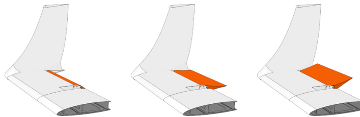
Figure 14.1: Tamarack active winglet with control surface [112]
