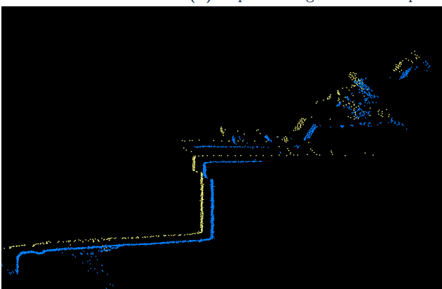
(c) Small (8 - 10cm) misalignment still present after trajectory correction in normal direction.
