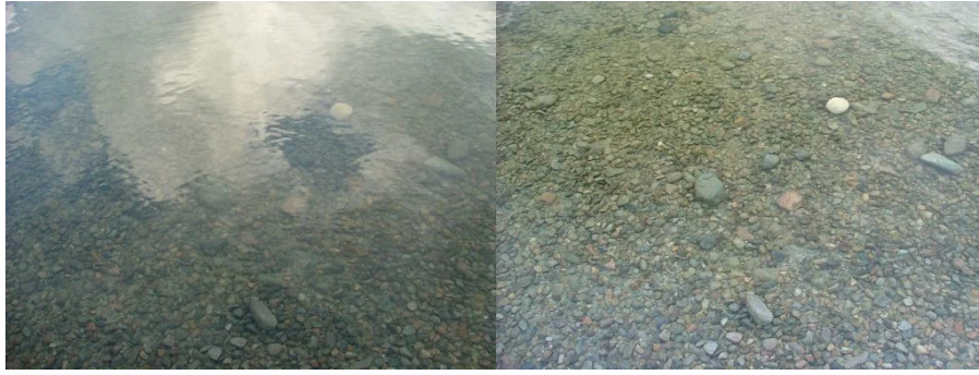
Figure 2.9: A body of water observed at Brewster's Angle. The photo on the left shows a significant amount of glare. The photo on the right is taken with a polarisation filter oriented normal to the plane-of-incidence, such that all reflected light — the glare — is filtered out, leaving only the light transmitted back through the water[16].
