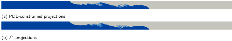
Figure D.5: Lock exchange: density field at the mesh at t^* = 10 using \ell^2 or PDE constrained particle-mesh projections. Note the different time scales used for the PDE-constrained projections and the local \ell^2 -projections.
