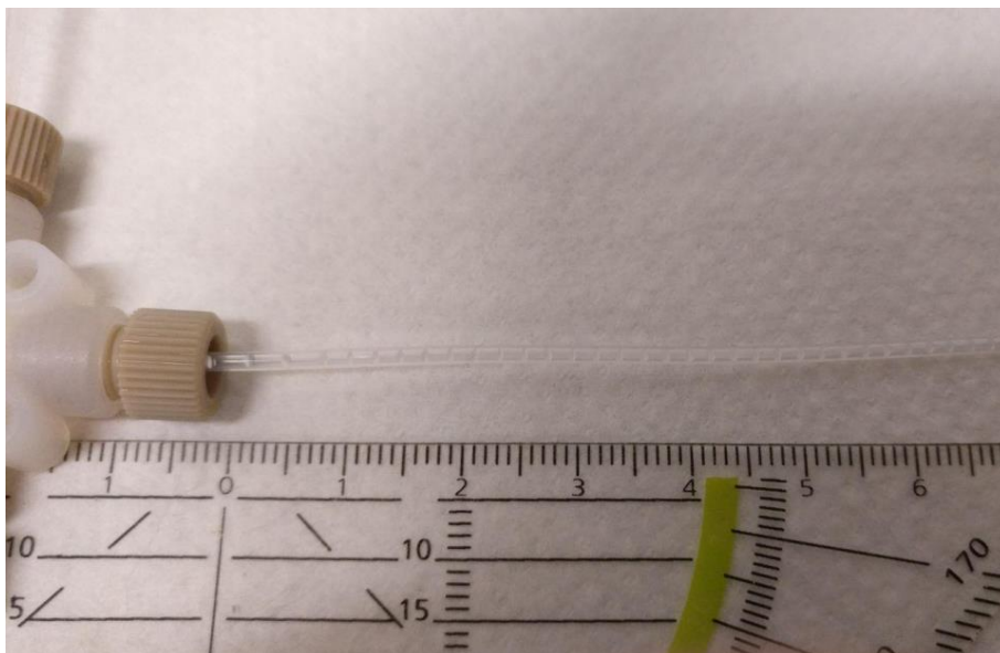
Figure 12 Image of the segmented flow at an oxygen liquid ratio of three to one at the beginning of the reactor.
