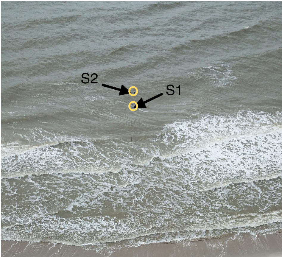
Figure 2: Locations of the echo sounders and pressure sensors, photographed from a drone during high tide. Four poles were installed during this field campaign, the data from the echo sounders and pressure sensors installed in the two offshore poles was used for this study. With the array facing approximately Northwest, this means the incoming wave direction is Southwest-west.
