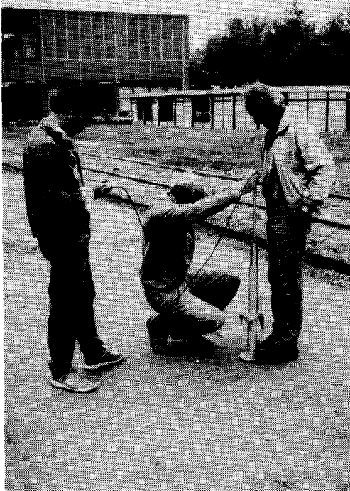
Figure 8.16: Clegg Impact Test in progress.
