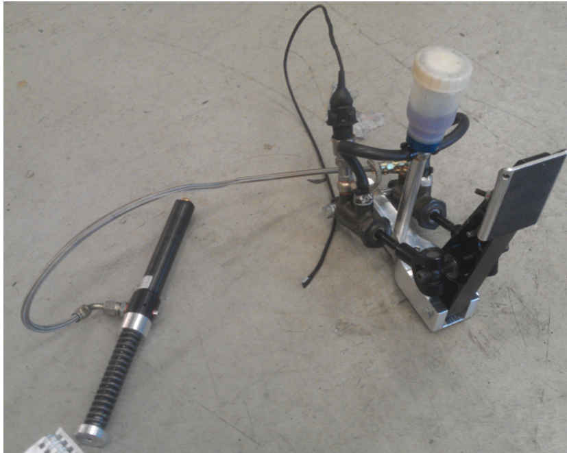
Figure 2.4: Complete brake pedal assembly.
