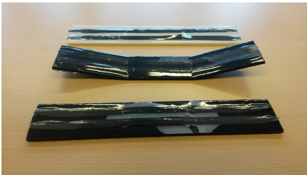
Figure 4. The grey rectangle on the top and the two black rectangles below it are the 3-D printed samples post fracture, placed on a sandstone-coloured desktop that forms the background. Top: ABS M30; middle: PC-ABS; bottom: nylon.
