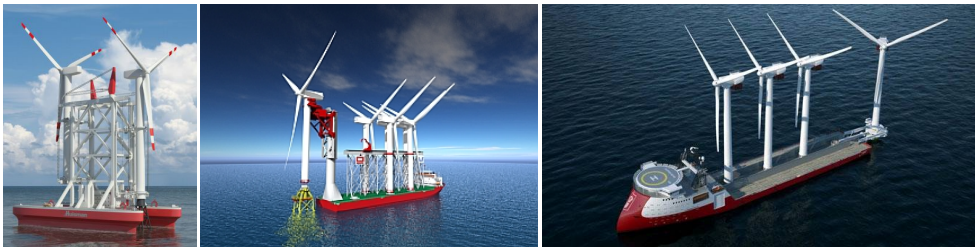
Figure 1.8: Dedicated turbine installation concepts; Huisman [l], IHC Vuyk [m], Ulstein [r]
