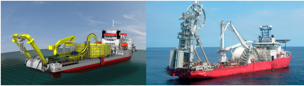
Figure 2.6: Left you see an illustration of a horizontal tensioner cable lay vessel, source: Germany: NSW Charters Cable Laying Vessel MV Aura. Right illustration you see a semi-vertical tensioner cable lay vessel, source: Subsea 7 reel-lay vessel seven Oceans.
