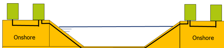
Figure 2.4: An interconnection between an offshore platform and an onshore structure. The cable is buried beneath the seabed
