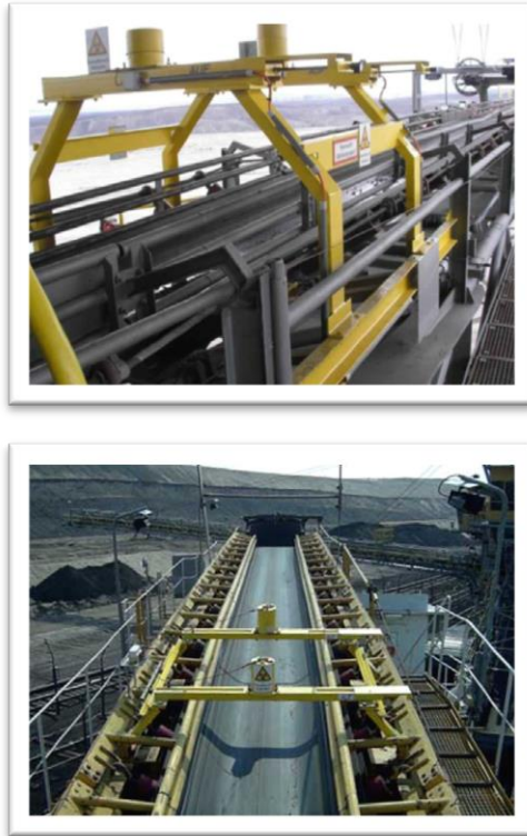
Figure 2.6: Radiometric sensor measurement device, installed on the conveyor belt, measuring blend of coal resulting from multiple excavators, just before the stock Pile (Source: MIBRAG)
