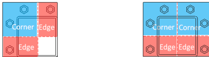
a) Layout of corner column splice (CCS). b) Layout of wall column splice (WCS).
