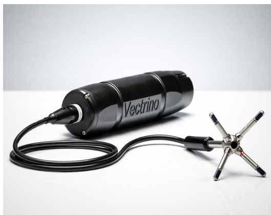
Figure 2.8: Acoustic Doppler Velocimeter (Adapted from Nortek AS, 2018).
