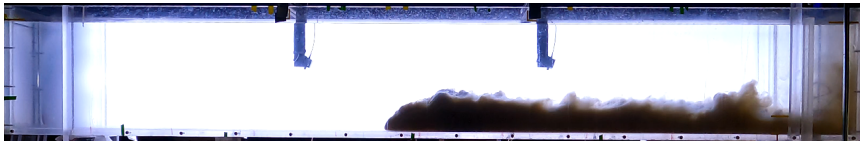
(b) Lock exchange flume during propagation of turbidity current
