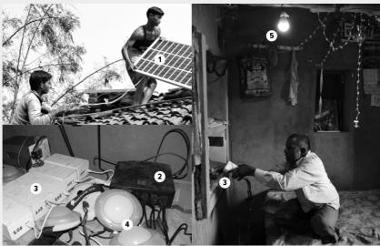
Figure 1: Energy exchange infrastructure and its components: solar panel (1), energy router (2), power banks (3), solar lamps (4), and a LED bulb connected to a power bank at a villager's home (5). Photographs: Abhigyan Singh.
