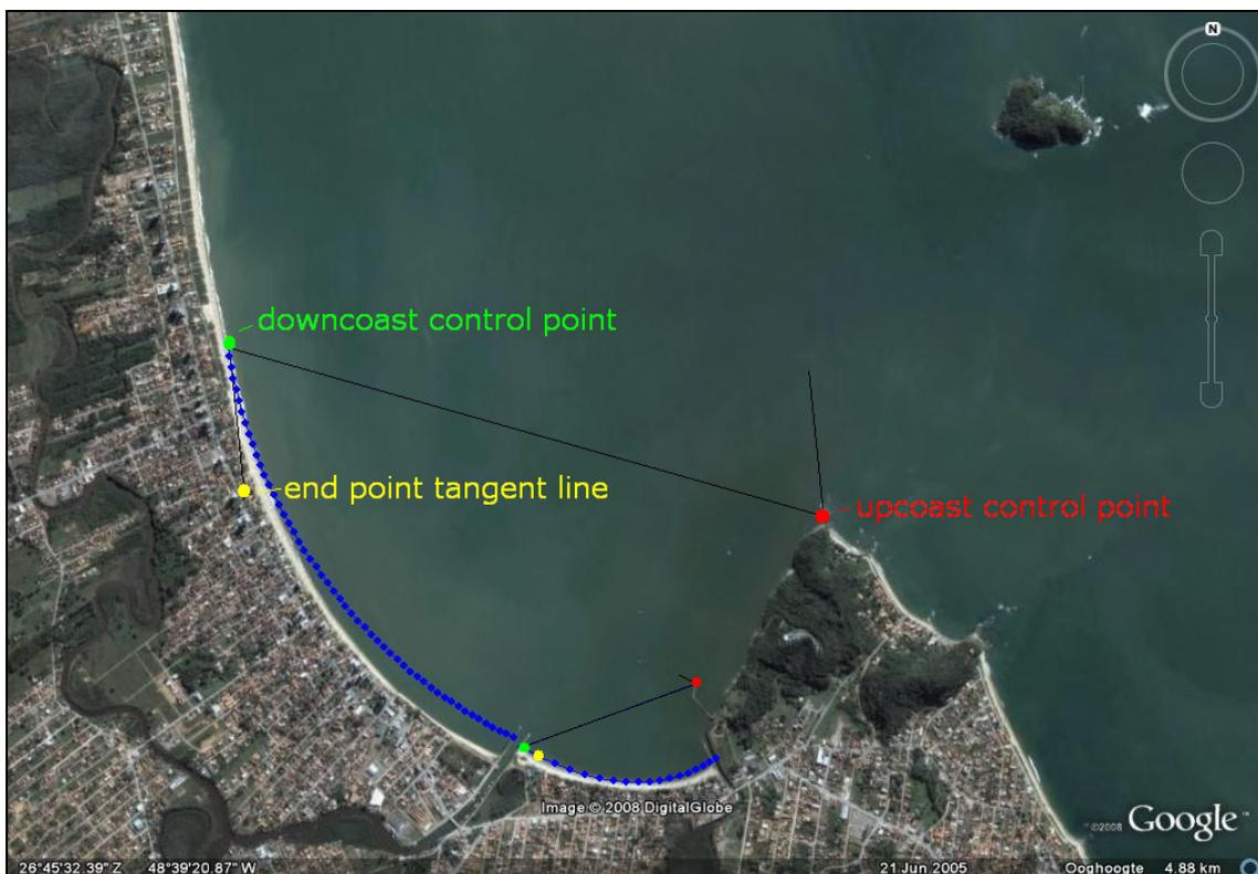
**Figure VIII - 5 Aerial photo of Piçarras beach with modeled beach planform in static equilibrium (alternative procedure)[16]**
