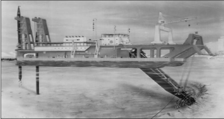
**Figure IX - 19 Image of a Cutter Suction Dredger**
