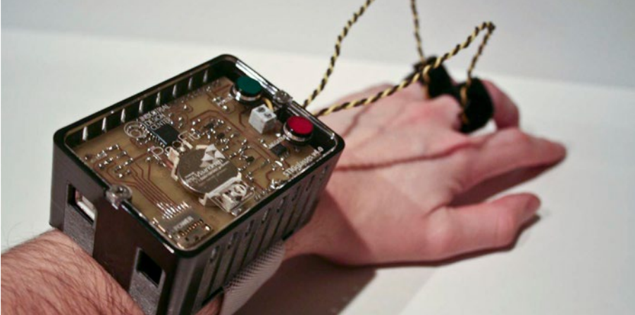
Figure 5. Arduino setup with EDA and valence event-mark buttons
