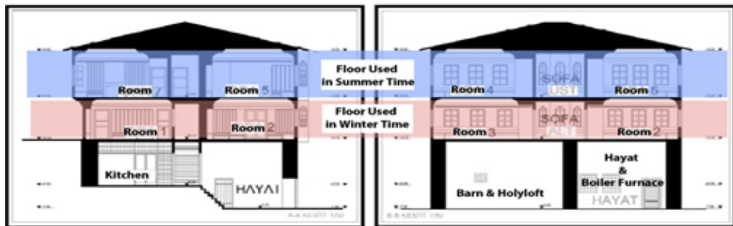
FIG. 10 Sections of Haci Huseyinler house and winter and summer time's parts. Sections of Haci Huseyinler house and winter and summer time's parts
