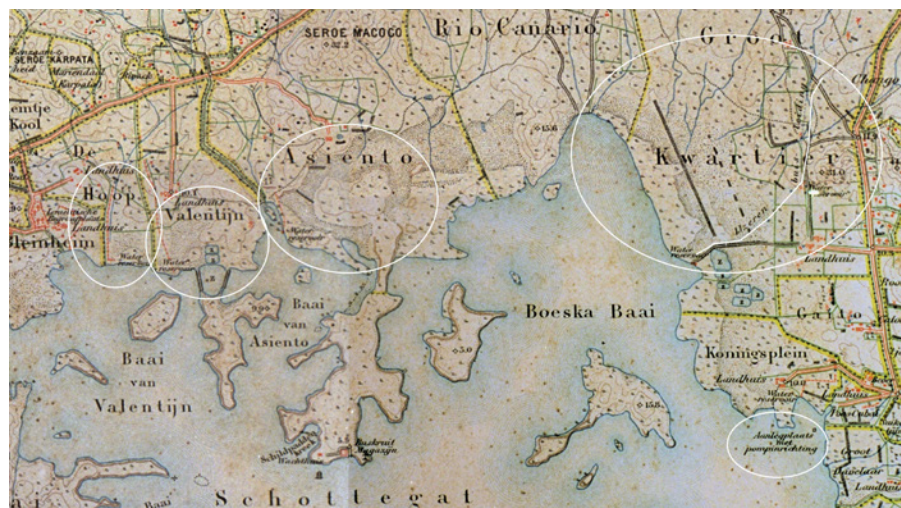
FIG. 16 This map shows the waterplantages around Schottegat bay. At Plantage Groot Kwartier an iron pipeline was constructed to direct water to the water reservoir on the shore of the bay. In 1911 Asiento only had three wind-powered wells. By 1918 there were 13 mills. Next to large earthen dams there are also soil storage waterreservoirs on the shore of the bay. In the east corner of this map there is a pumpingstation. Most probably for pumping water into cargo ships.
