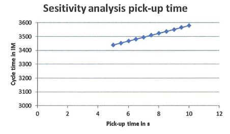
Figure 5.18: Sensitivity analysis of pick-up time and its influence on the total cycle time.
