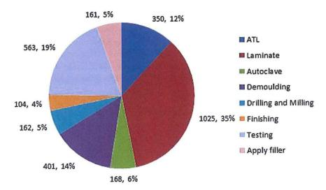
Figure 3.5: Process times of main processing steps for the production of the inboard flap shells.
