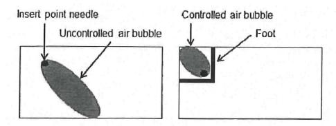
Figure 5.10: Peel initiation with and without using a foot to guide the airflow.
