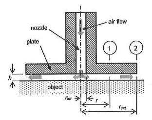
Figure 4.13: Working principle of Bernoulli gripper.
