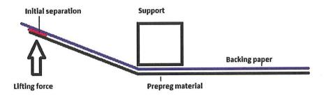
**Figure 4.23:** Principle of initial separation of backing paper by controlled mechanical bending.
