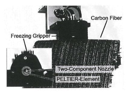
Figure 4.15: Hydro adhesive gripper with Peltier element.
