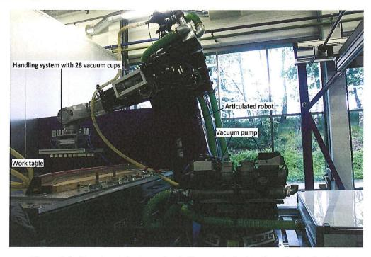
Figure 6.1: Experimental set-up of end-effector attached to the articulated robot.
