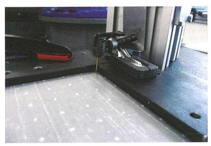
Figure 6.6: Positioning of injection needle before peel initiation.
