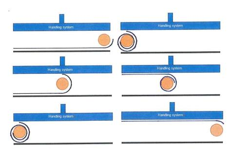
Figure 5.13: Removal strategy of backing paper from upper side of prepreg.
