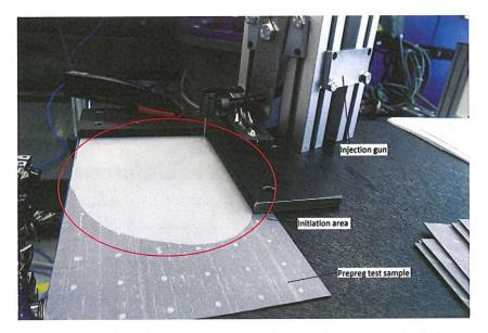
Figure 6.7: Initiation area on prepreg after injection of pressurized air.
