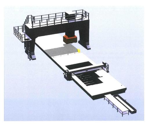
**Figure H.1:** Overview of the robotic cell lay-out with ATL, ATL lay-up table, integrated bridge and lay-up table.
