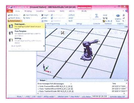
**Figure L.2:** Example of adding a virtual controller to the robotic cell to control the movements.
