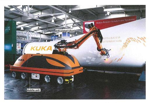
Figure 4.8: Articulated robot placed onto a mobile unit.
