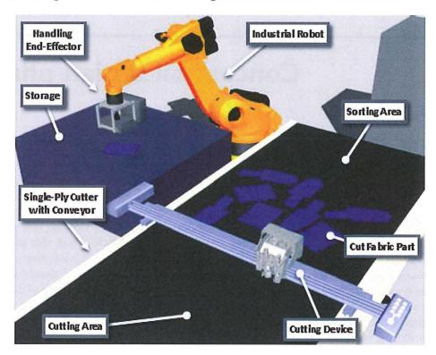
Figure 4.1: Robotic cell lay-out of an articulated robot at fixed place next to cutting table.
