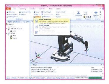
Figure L.3: Example of creating a workobject or reference system.
