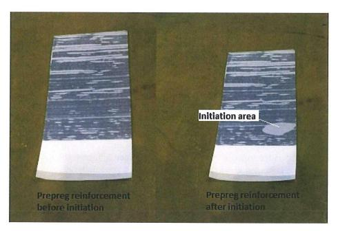
**Figure 4.25:** Small experiment performed to proof peel initiation concept. With test sample before peel initiation area on left hand side and initiated area on right hand side.
