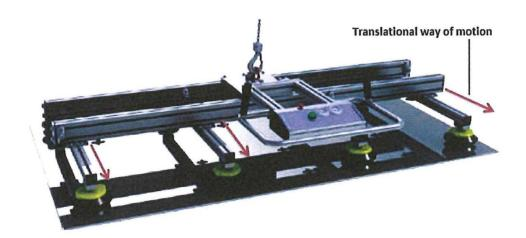
Figure 4.20: Gripper with retractable bars, where end-effectors can be individually actuated.
