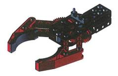
Figure 4.11: Example of a mechanical gripper.
