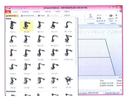
Figure L.1: Example of import of industrial robot, linear track unit or other CAD models.
