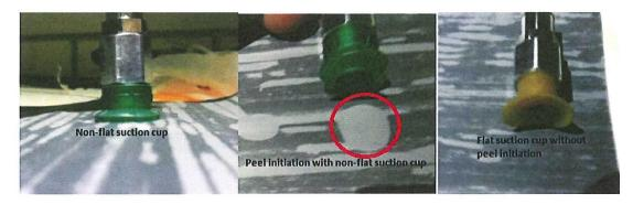
Figure 5.9: Affected initiation area by using non-flat and flat suction cup.
