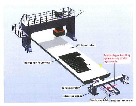
**Figure 6.4:** Simulation of robotic cell in ABB robot studio showing positioning of integrated bridge and handling system on top of side lay-up table.
