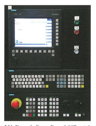
Figure 5.14: Picture of a Siemens Sinumerik 840D control system.
