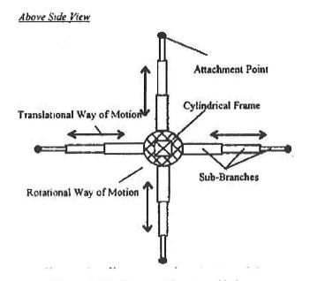
Figure 4.19: Gripper with retractable bars.
