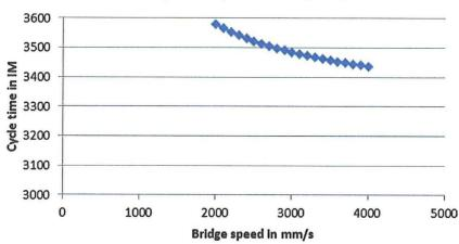
**Figure 5.21:** Sensitivity analysis of travelling speed of the integrated bridge and its influence on the total cycle time.
