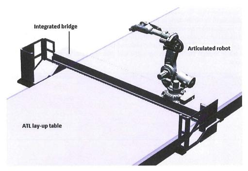
**Figure 4.6:** Integrated bridge attached to ATL lay-up table with articulated robot placed on top.
