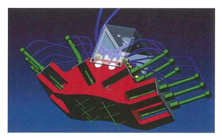
Figure 4.14: Working principle of needle Gripper with twelve needles.
