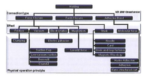
Figure 4.10: Overview of different end-effectors types.
