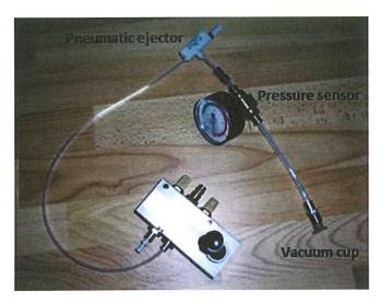
Figure 5.7: Trial set-up of ejector and vacuum cup.
