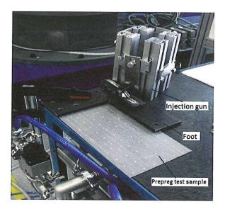
Figure 6.5: Peel initiation test set-up of injection gun and prepreg test sample.
