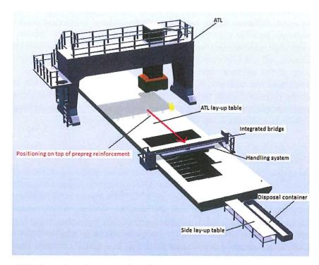
**Figure 6.2:** Simulation of robotic cell in ABB robot studio showing pick-up of prepreg from ATL lay-up table.
