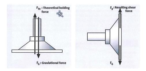
Figure 5.4: Two lifting cases for gripping by vacuum suction.
