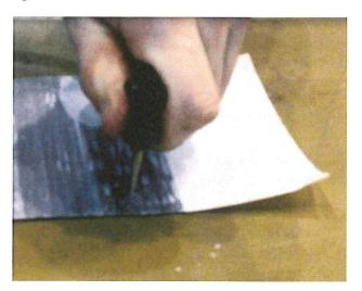
**Figure 4.22:** Principle of peel initiation by injecting compressed air with an injection needle between the backing paper and prepreg material.
