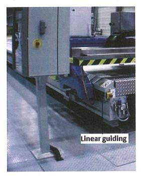
Figure 5.2: Linear guiding of integrated bridge, integrated in the ATL lay-up table.
