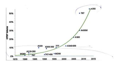
Figure 1.1: Development of carbon fibre reinforced plastic in aircrafts.
