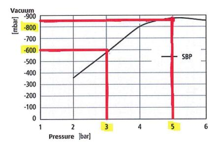
Figure 5.8: Relation applied pressure and generated vacuum pressure for air-tight materials.
