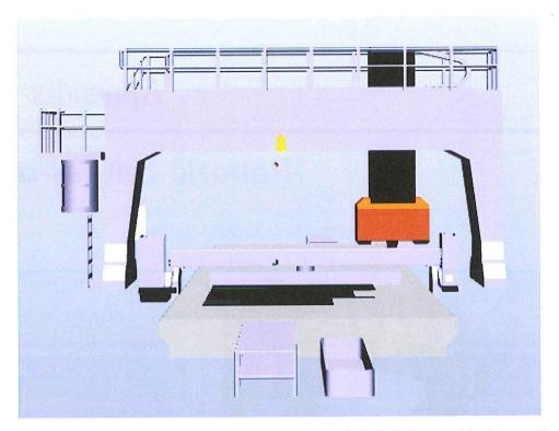
**Figure H.2:** Frontview of the robotic cell lay-out with ATL, ATL lay-up table, integrated bridge and lay-up table.
