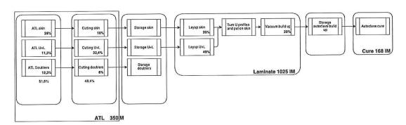
Figure 5.16: Work breakdown of ATL, laminating and curing step.
