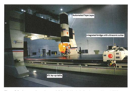
**Figure 3.2:** Automated tape layer on left hand side, including lay-up table and CNC cutter on the right hand side.
