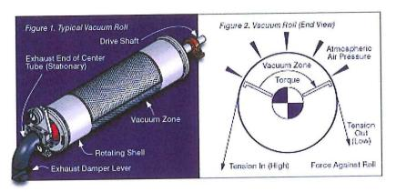
Figure 5.11: Lay-out of vacuum roll.
