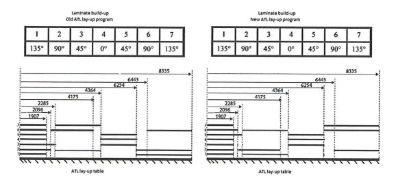
**Figure 5.15:** Change of ATL program in order for not flipping the prepreg material anymore during stacking. ATL program with flipping is shown on left side and for the new case on the right side.
