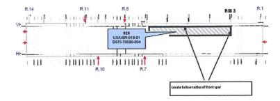
Figure D.18: Eighteenth step in skin build-up of lower shell.
