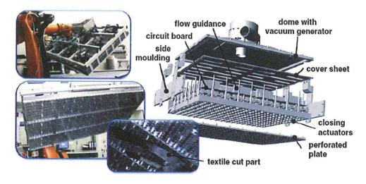
Figure 4.18: Multi acuator vacuum system.
