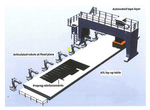
Figure 4.2: Multiple articulated robots at fixed place along the entire length of the ATL.
