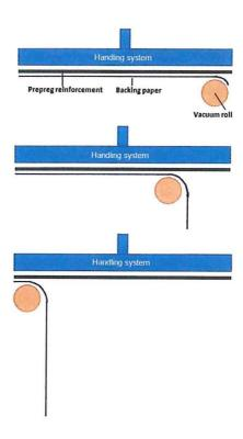
Figure 5.12: Removal strategy of backing paper from lower side of prepreg.
