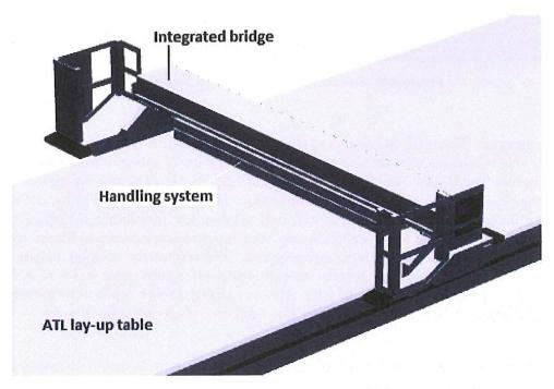
Figure 4.7: Integrated bridge attached to ATL lay-up table with integrated handling system.
