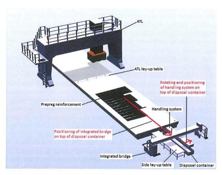
**Figure 6.3:** Simulation of robotic cell in ABB robot studio showing positioning of integrated bridge and handling system on top of disposal container.
