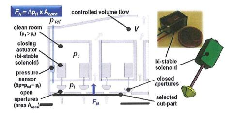
Figure 5.3: Concept of the selective gripping technology.
