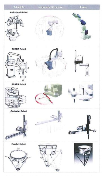
Figure 4.9: Overview of industrial robots principles and kinematic structure.
