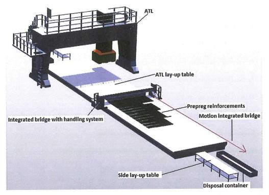
Figure 5.1: Overview of the robotic cell lay-out with ATL, ATL lay-up table, integrated bridge and lay-up table.
