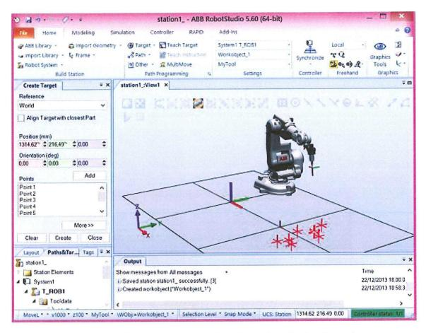
Figure L.4: Example of creation of targets which will be the basis for the robot path.
