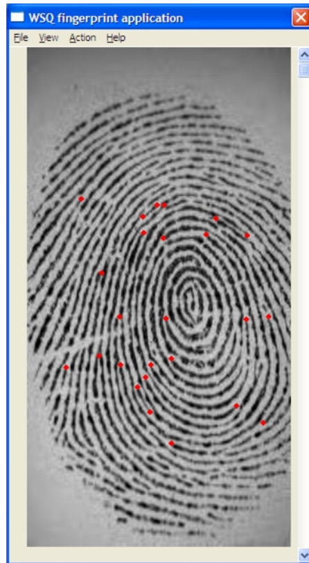
Figure 6.4: Application showing a fingerprint image with minutiae computed by the MINDTCT system
