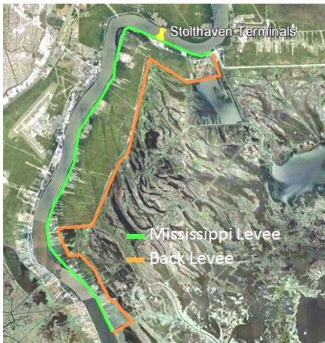
Figure 3-2 Existing levee system around the terminal
