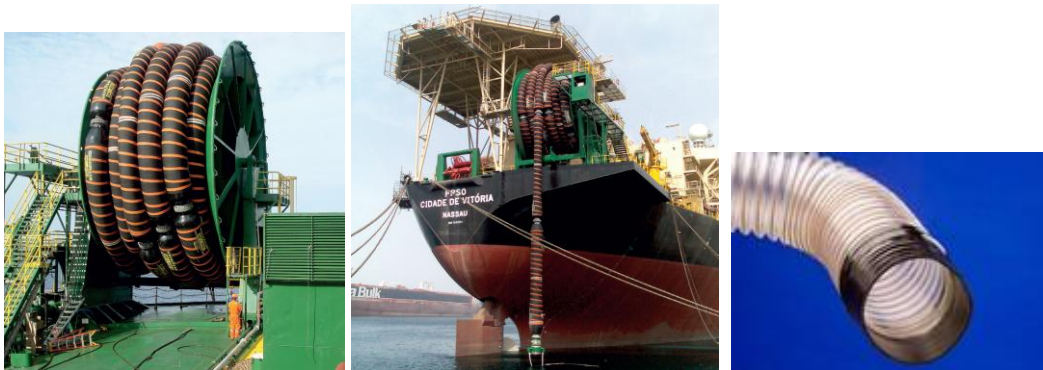
Figure 8-23 [left & mid] Example of flexible pipelines of tanker loading systems 13 ; [right] Example of flexible and compressible pipelines 14
