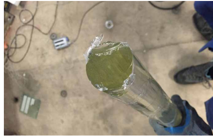
FIG. APP.A.17 Fractured face of glass rod
