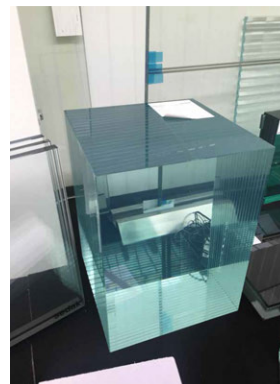
FIG. 2.24 20 x 12mm low iron glass with VLT=57%*
