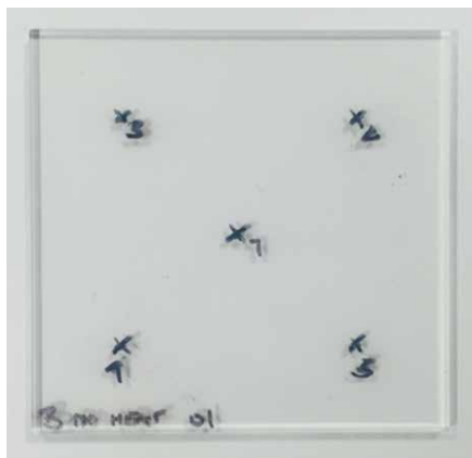
FIG. 5.17 Test specimen with measuring points
