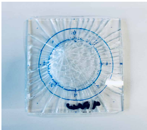
FIG. 6.44 Fracture Pattern specimen 4 AR
