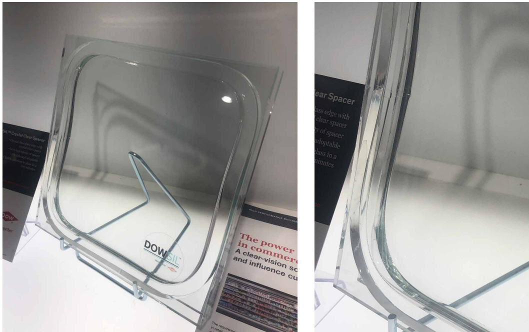
FIG. 7.37 Transparent Glass edge seal presented by DowSil, as seen at Glass Performance Days, Tampere 2019
