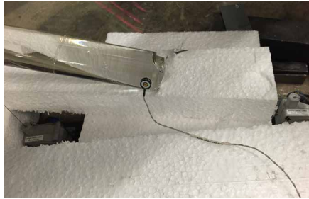
FIG. APP.A.16 Fractured glass rod
