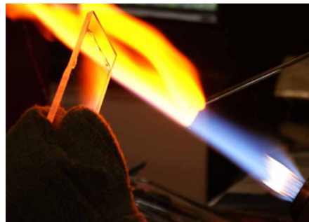
FIG. 6.9 'Additive' manufacturing of thin glass layers on 50mm x 200mm flat glass - Due to the absence of a 3D printing process for glass at the time the experiments were carried out, this connection was chosen to mimic an additive manufacturing process and verify the possibility of connecting thinner layers of glass.
