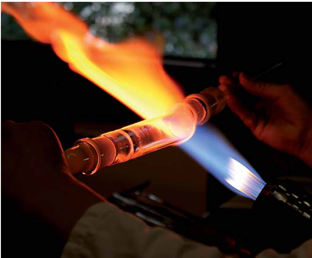
FIG. 5.1 Glass laboratory ware heat bonded connection
