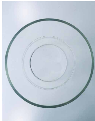
FIG. 5.5 Welded glass tube fabricated by Schott
