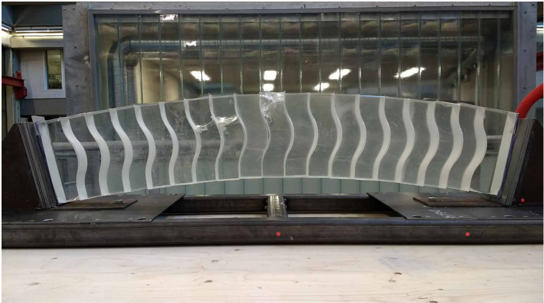
FIG. 3.71 Interlocking cast glass brick footbridge (Snijder, TU Delft)
