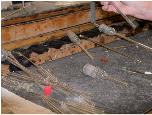
FIG. 5.2 Glass tube ends used to allow the manual handling of tubes
