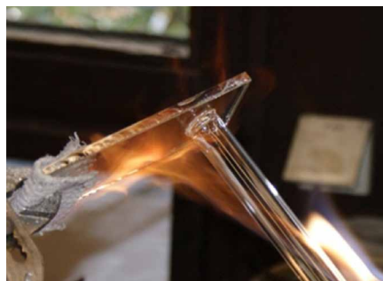
FIG. 6.6 20mm tube (2mm wall thickness) attached to 50 x 200mm flat glass. - Tubular sections are commonly used in scientific glass blowing, so a tube with a small radius and wall thickness was chosen to continue feasibility studies on the manufacturing of the connections.
