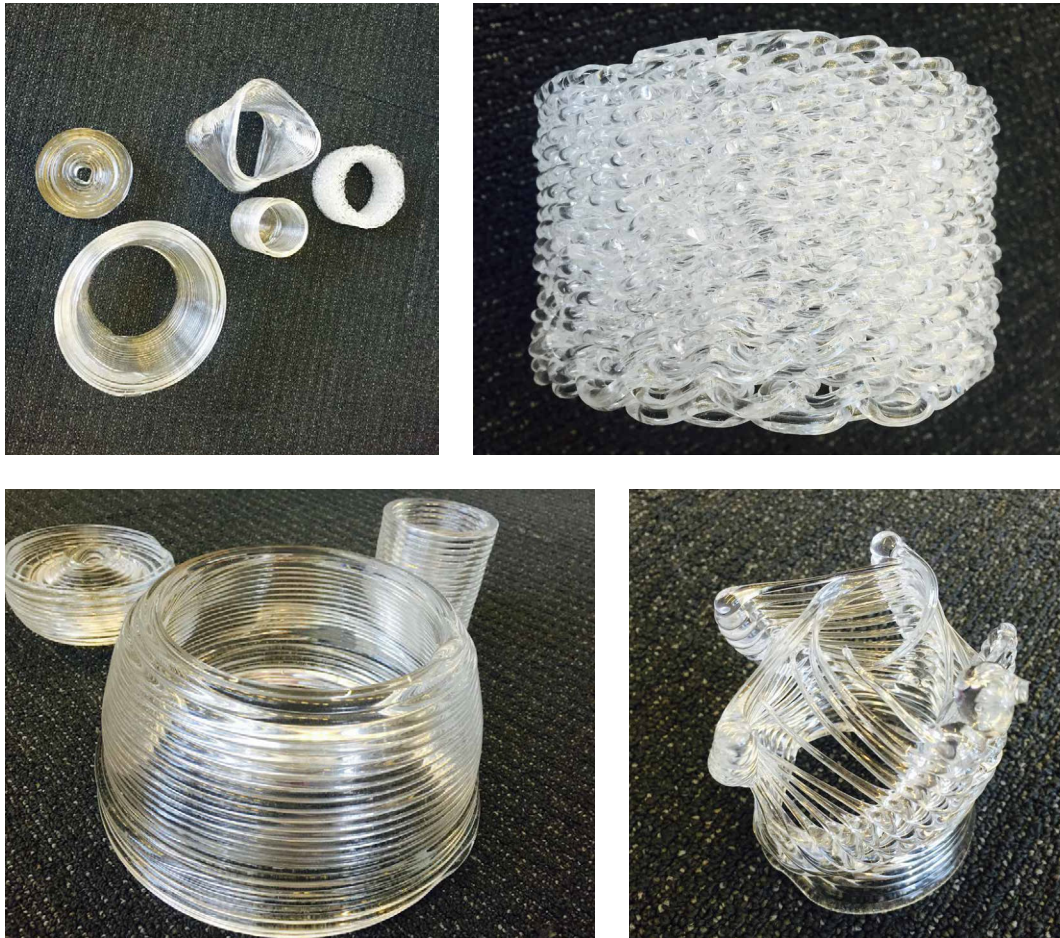
FIG. 5.6 Examples of objects created with 'G3DP' process at MIT
