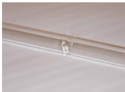
FIG. 6.4 Butt joint of two 40mm tubes (2mm wall thickness). - This connection was selected as it is a common connection crafted in the manufacture of laboratory ware and it could be assessed in flexure comparing to an AR tube with the same dimensions.
