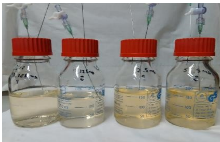
Figure 3.15: Coloured solution due to the iron oxidation/bromate reduction in presence of nitrate at 72 hours.
