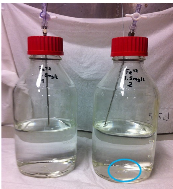
Figure C.12: Imperceptible coloration of solution but small floc formation with the 0.03 mM iron dose during the bromate ( 60 \mu\text{g/L} ) and nitrate ( 10 \text{ mg/L} ) reduction after 5 days.
