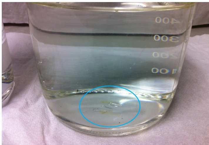
Figure C.13: Zoom to the floc formation with the 0.03 mM iron dose during the bromate ( 60 \mu\text{g/L} ) and nitrate ( 10 \text{ mg/L} ) reduction after 5 days.
