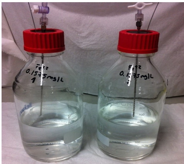
Figure C.11: Imperceptible change of colour with the iron dose 0.007 mM during bromate ( 60 \mu\text{g/L} ) and nitrate ( 10 \text{ mg/L} ) reduction after 5 days.
