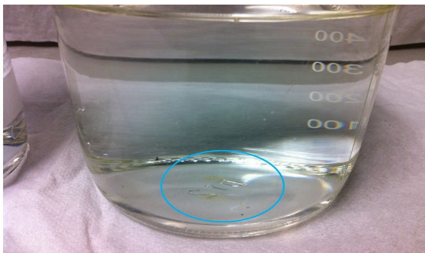
Figure 3.21: Zoom to floc formation during the reaction of 0.03mM iron and bromate (60ug/L) and nitrate (10mg/L) after 5 days.
