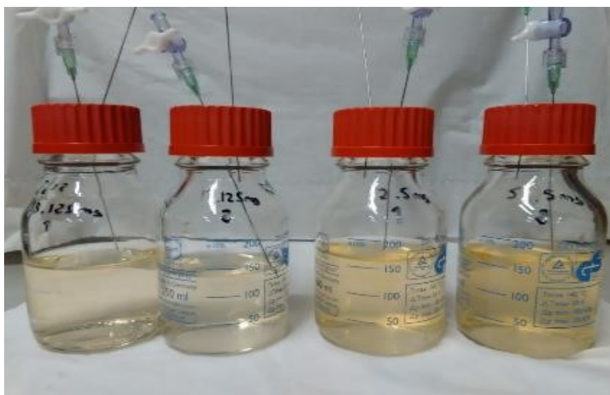
Figure C.8: Coloured solution due to the iron oxidation/bromate reduction in presence of nitrate at 2 hours.
