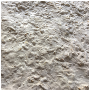
Mycelium Composite Wheat
