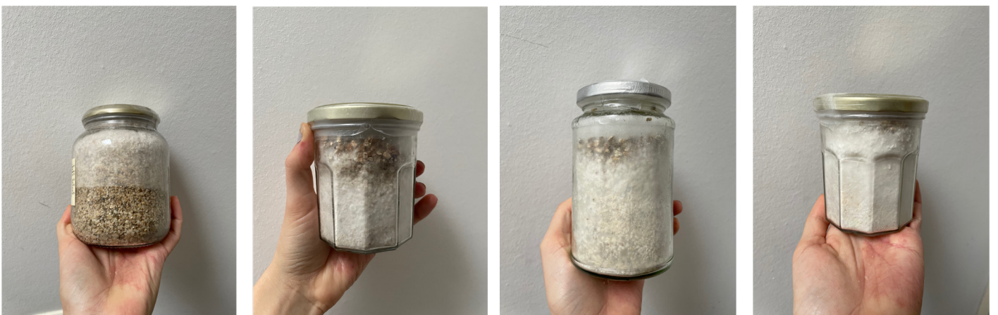
Figure 25 | Mycelium Processing Experiment | Complete Grain Spawn Growth of Mycelium
