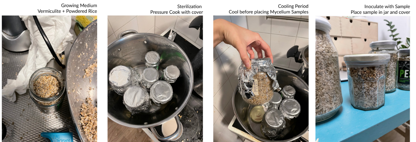
Figure 24 | Mycelium Processing Experiment | Steps for Starting Mycelium Growth in Growing Medium
