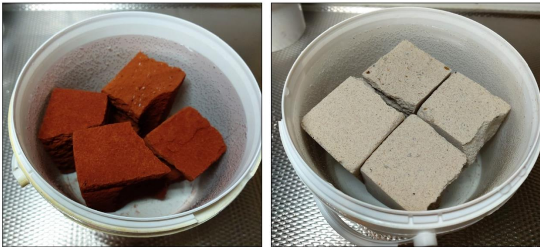
Picture 64: shows the used bricks samples for initial terrarium testing, soaked in water (own picture)
