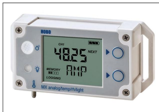
Picture 83: Hoboware MX1104 measuring device (own picture)
