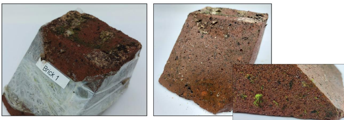
Picture 78: Redbrick sample one, before and after the removal of the plastic wrapping (own picture)
