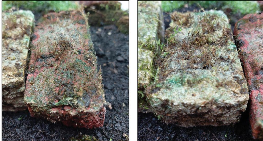
Picture 87: Brick sample from initial terrarium test, moss browning due to high temperature in the terrarium (own picture)
