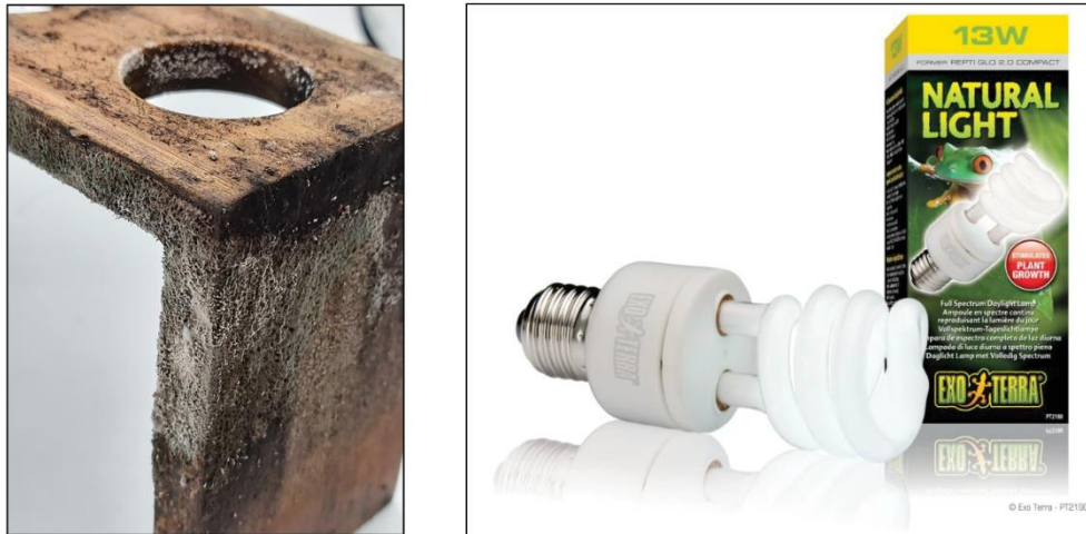
Picture 90: Left: microorganism growth on the wooden table (own picture) and right: the used growth lamp for the glass terrarium test, picture retrieved from: http://www.exo-terra.com/nl/products/natural_light.php
