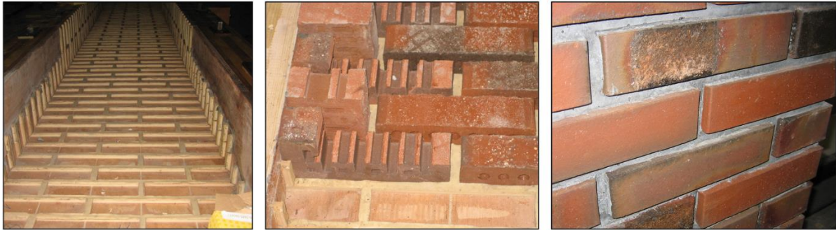
Image 34: shows how prefabricated masonry facade element is made, images provided by Dr. Roel Schipper (Source: wall elements for Maasstad Ziekenhuis Rotterdam fabricated by Loveld, www.loveld.com )
