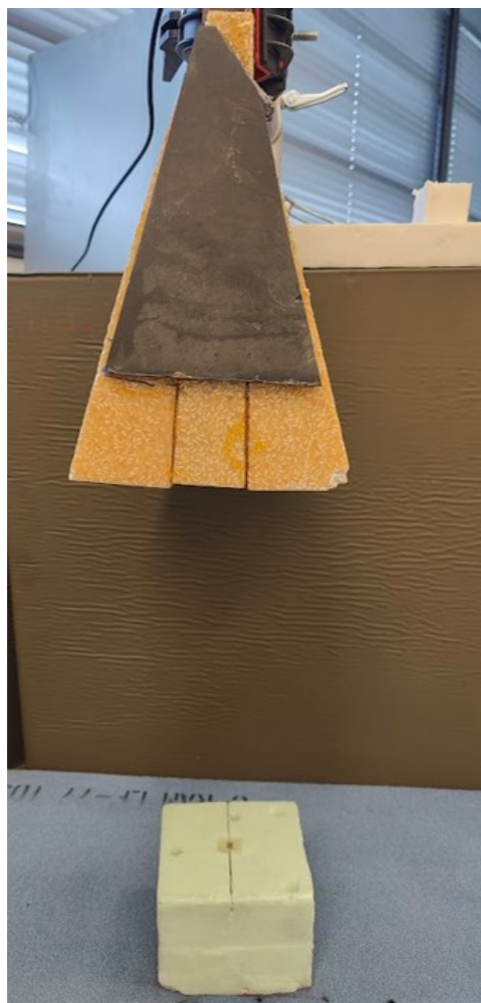
Figure 4.11: Horn antenna set up with the sensor
