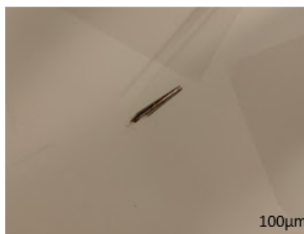
Figure 3.6: Curling of the structure seen after removing from the acetone bath
