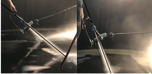
Figure 6: Relationship between pitch angle and nozzle deflection.
