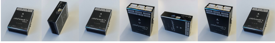
Figure 5.2: Bank angle verification scheme; the PX4 Autopilot was (i) rolled by 90°, (ii) rolled back, (iii) pitched up by 90°, (iv) yawed by 90°, and finally (v) yawed and (vi) pitched back into its original position
